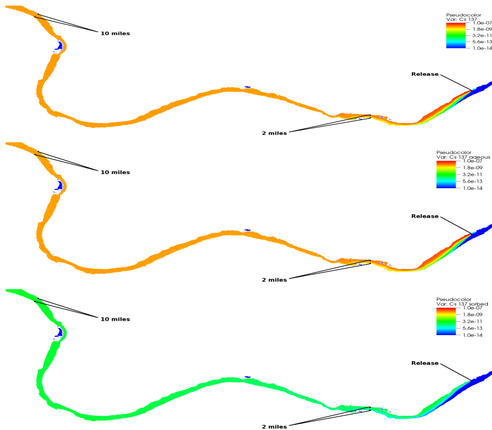
Figure 5-13. Simulated Small River ^{137}\text{Cs} Water Column Concentrations ( \text{Bq}/\text{m}^3 ) in the Aqueous-Only Simulation (top), Aqueous Phase in the Sediment-Inclusive Simulation (middle), and Suspended Sediment-Sorbed Phase in the Sediment-Inclusive Simulation (bottom). Flow is from right to left. Downstream blue-colored areas are inundated but not directly connected to the channel. The figures extend approximately 10 mi below the release location. Black markers indicate sample locations 2 and 10 mi downstream.
