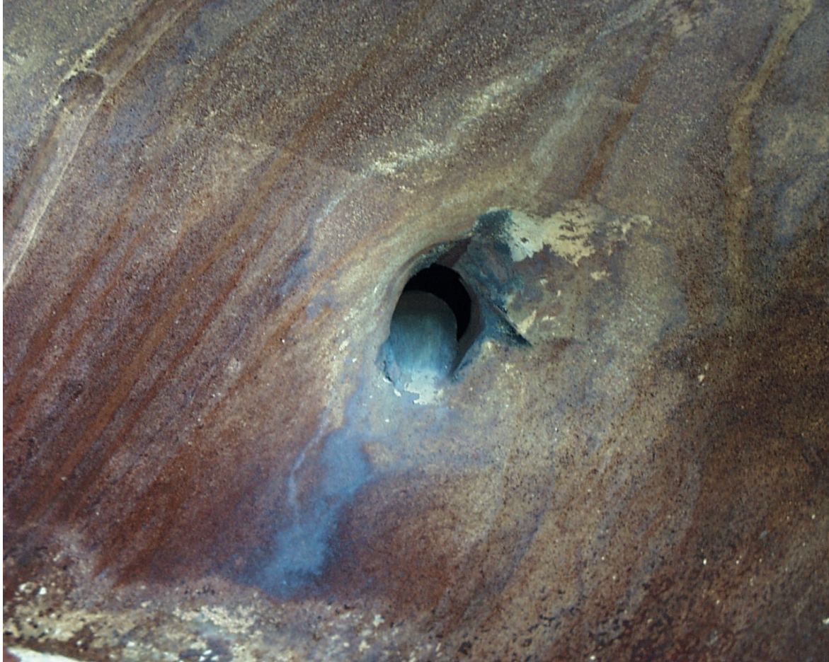
Figure 5.3. Puncture in Tank Car
