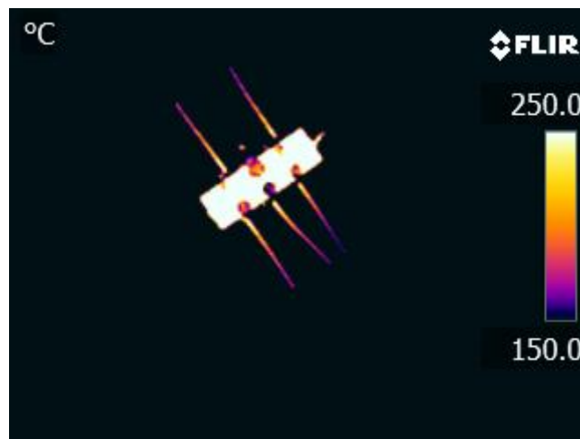
Figure 4-13. Thermal image of XLPE wires following a 60.0 minute heating ramp and a 5.0 minute soak period
