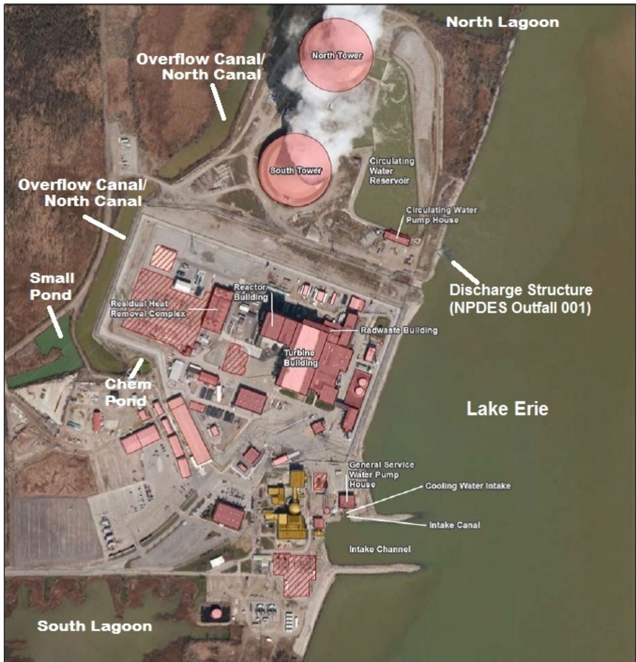
Figure 3-5. Fermi 2 Cooling Water Supply Facilities and Major Surface Water Features
