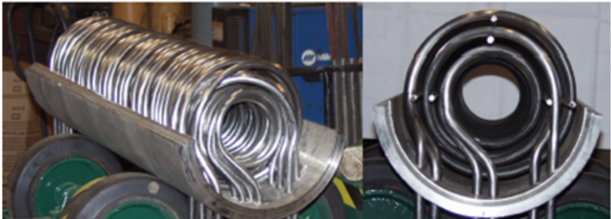
Figure 8 Helical Coil SG Bundle Photo [18,19,34]
