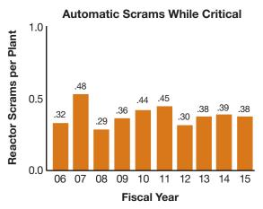
A reactor is considered "critical" when it achieves a self-sustaining nuclear chain reaction, such as when the reactor is operating. The sudden shutting down of a nuclear reactor by the rapid insertion of control rods, either automatically or manually by the reactor operator, is referred to as a "scram." This indicator measures the number of unplanned automatic scrams that occurred while the reactor was critical.
