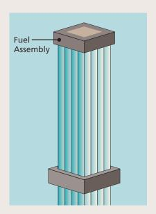
After 5-6 years, spent fuel assemblies (which are typically 14 feet [4.3 meters] long and which contain nearly 200 fuel rods for PWRs and 30–100 fuel rods for BWRs) are removed from the reactor and allowed to cool in storage pools. At this point, the 900-pound (409-kilogram) assemblies contain only about one-fifth the original amount of uranium-235.
