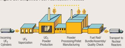
Figure 29. Simplified Fuel Fabrication Process
