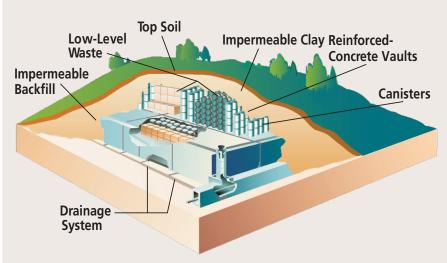
Figure 30. Low-Level Radioactive Waste Disposal
