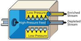
membrane or vessel than do heavier isotopes.) This process involves filtering UF $_6$  gas to separate uranium-234 and uranium-235 from uranium-238, increasing the percentage of uranium-235.
