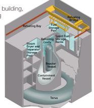
continuous cooling for the fuel, and provide shielding from the radioactive spent fuel. The process is reversed when fuel is removed from the fuel pool and placed in the reactor. In BWRs the fuel remains in a vertical position throughout the process.
