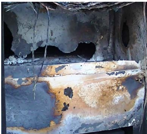
(c) Cabinet 7 Vertical Bus Bar Location
