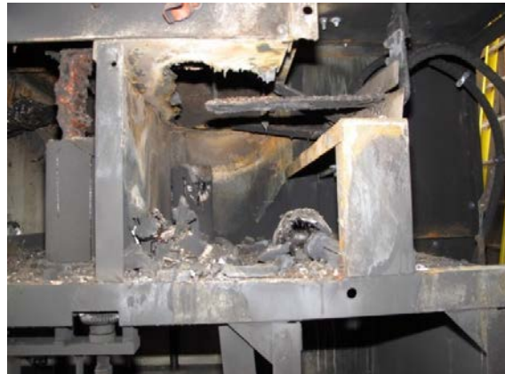
Figure 5.6-6. SWGR Test 5 Insulator and Bus Bar Damage
