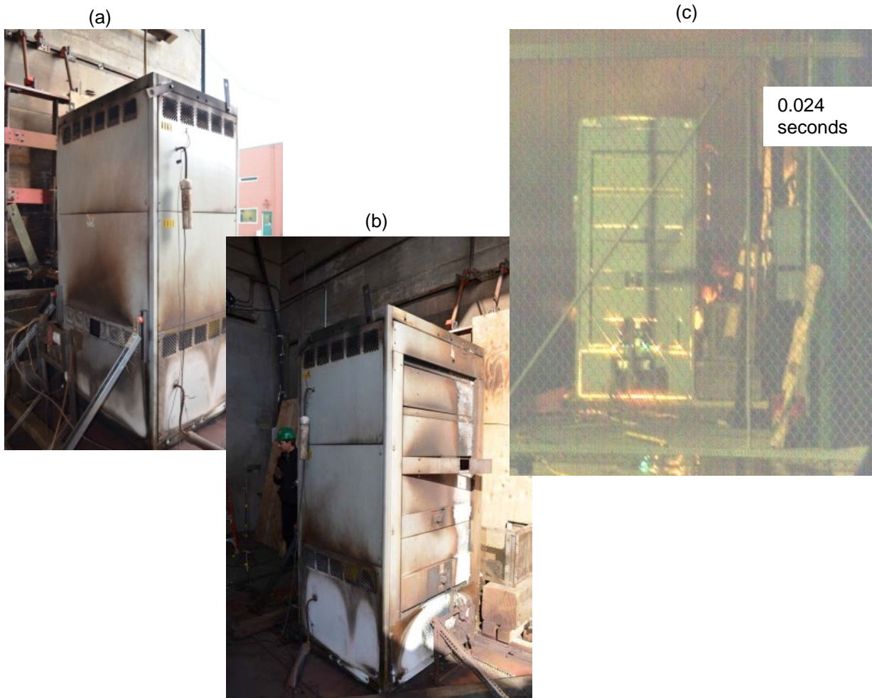
Figure 2.10-3. DP Test 3 Exterior Cabinet Damage
