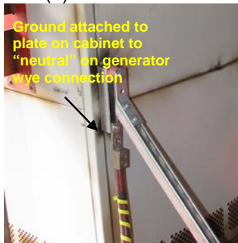
Figure 2.11-7. DP Test 4 Ground Fault during the Arc
