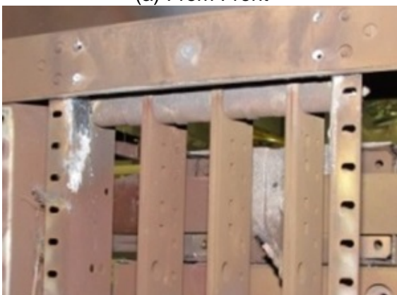
Figure 2.11-8. DP Test 4 Bus Bar Damage at Arc Location
