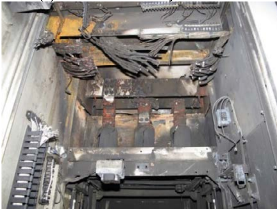
Figure 5.6-6. SWGR Test 5 Insulator and Bus Bar Damage
