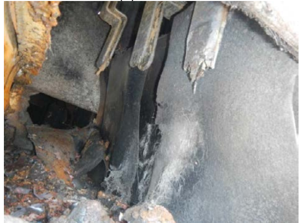
Figure 4.9-3. SWGR Test 2 Insulator and Bus Bar Damage
