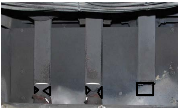
Figure 7.2-7. SWGR Test 6 Arc 1, Cabinet 7 Bus Bar Damage
