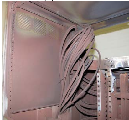
Figure 2.12-5. DP Test 5 Interior and Cable Damage
