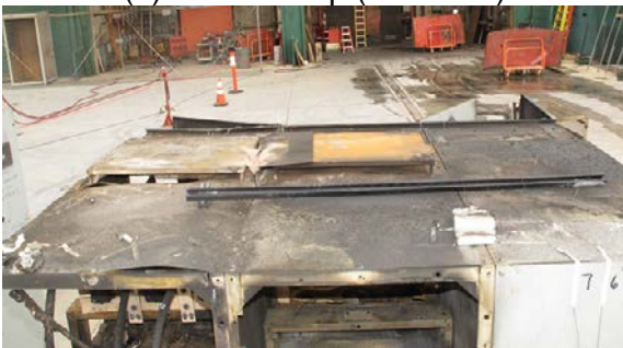
Figure 5.6-3. SWGR Test 5 Exterior Damage
