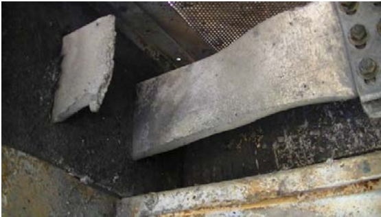
Figure 7.2-4. SWGR Test 4 Arc 2, Cabinet 7 Bus Bar Damage
