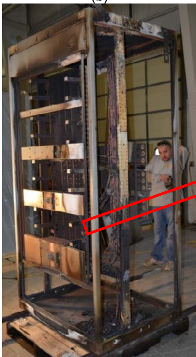
Figure 2.8-4. DP Test 1 HEAF and Fire Interior Damage
