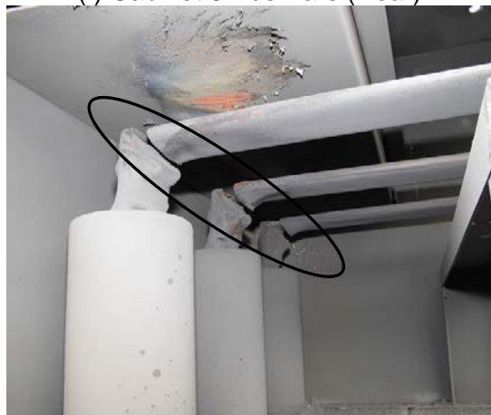
Figure 5.5-6. SWGR Test 4 Insulator and Bus Bar Damage
