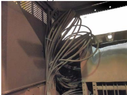
Figure 2.12-5. DP Test 5 Interior and Cable Damage
