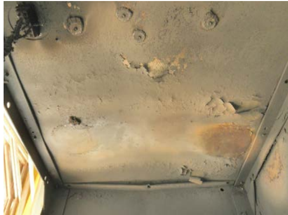
Figure 5.7-12. SWGR Test 6 Arc 2, Breaker Secondary Side Damage
