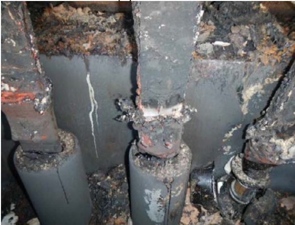
Figure 4.9-3. SWGR Test 2 Insulator and Bus Bar Damage
