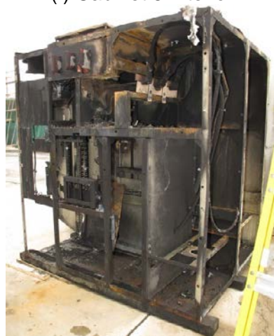
Figure 5.6-5. SWGR Test 5 Interior Damage, Detailed
