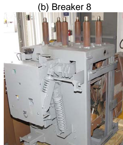
Figure 5.7-13. SWGR Test 6 Breaker 8 Damage
