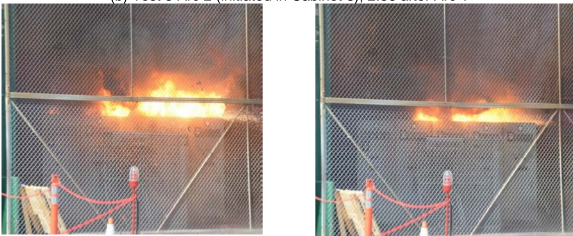
Figure 5.6-1. SWGR Test 5 Arcs
