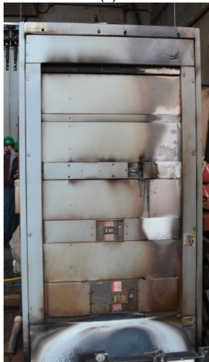
Figure 2.8-3. DP Test 1 Exterior Damage
