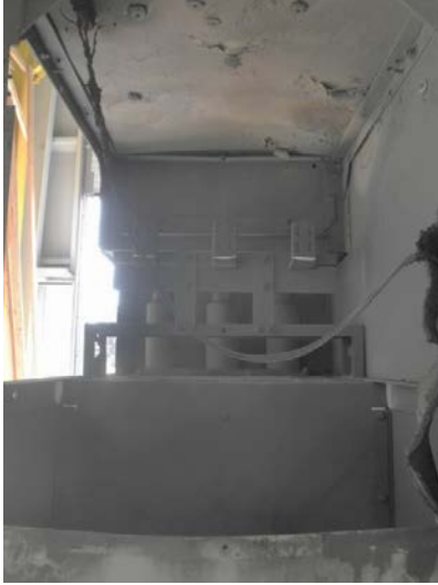
Figure 5.7-12. SWGR Test 6 Arc 2, Breaker Secondary Side Damage
