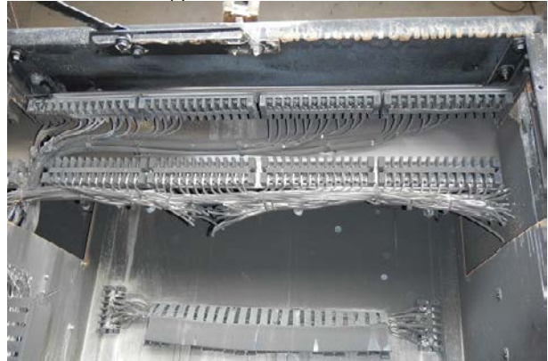
Figure 4.9-2, continued. SWGR Test 2 Interior Damage
