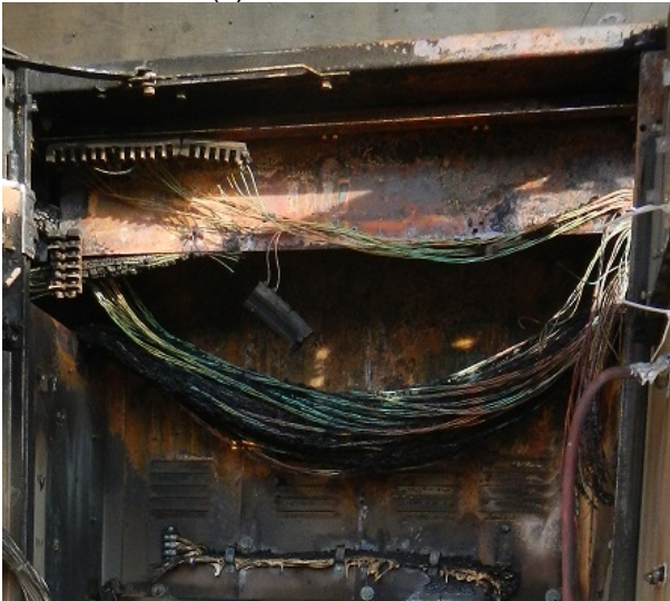
Figure 4.9-2. SWGR Test 2 Interior Damage, Continued
