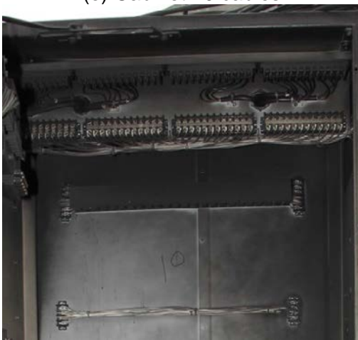
Figure 5.6-5. SWGR Test 5 Interior Damage, Detailed
