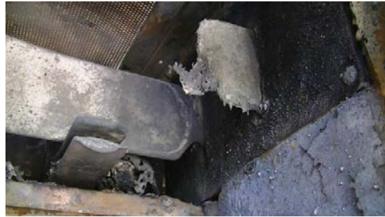
Figure 7.2-4. SWGR Test 4 Arc 2, Cabinet 7 Bus Bar Damage
