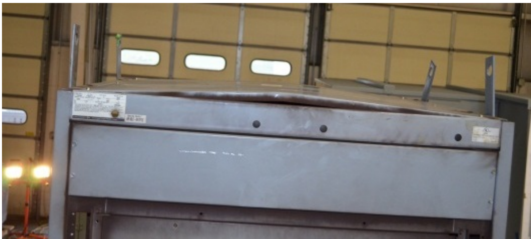
Figure 2.9-3. DP Test 2 Cabinet Top Deformation
