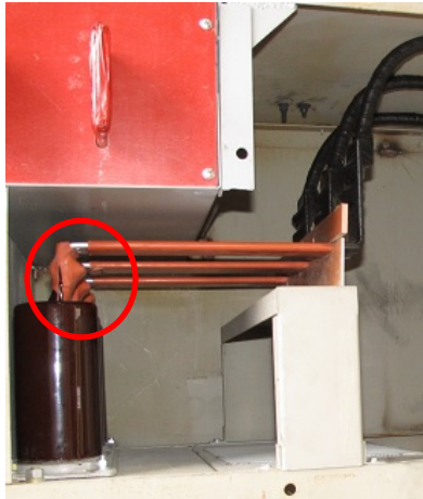
Figure 7.2-6. SWGR Test 5 Arc 2, Cabinet 8 Rear Bus Bar Damage
