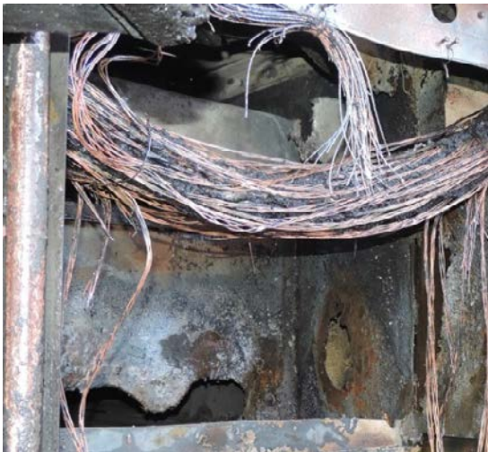
Figure 7.2-3. SWGR Test 4 Arc 1, Cabinet 7 Bus Bar Damage
