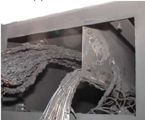
Figure 5.5-5. SWGR Test 4 Interior Damage, Detailed
