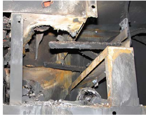
Figure 7.2-6. SWGR Test 5 Arc 2, Cabinet 8 Rear Bus Bar Damage
