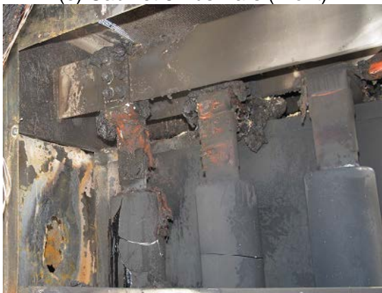
Figure 5.5-6. SWGR Test 4 Insulator and Bus Bar Damage
