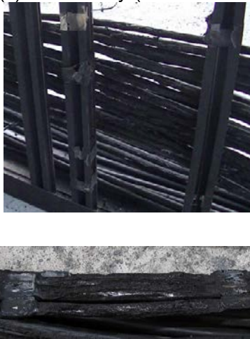
Figure 5.5-3. SWGR Test 4 Exterior Damage
