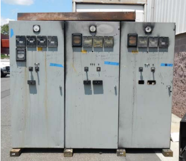
Figure 4.10-3. SWGR Test 3 Exterior Damage
