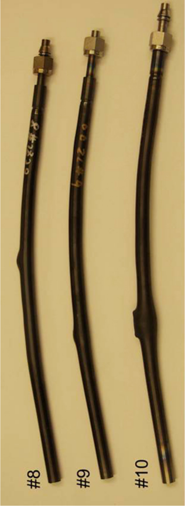
Figure E.1: Post-4-PBT images of ramp-to-rupture samples from OCZL#8, #9, and #10 test samples, which were pressurized at 300°C to 600, 400, and 1600 psig, respectively, heated to rupture, and cooled without quench.
