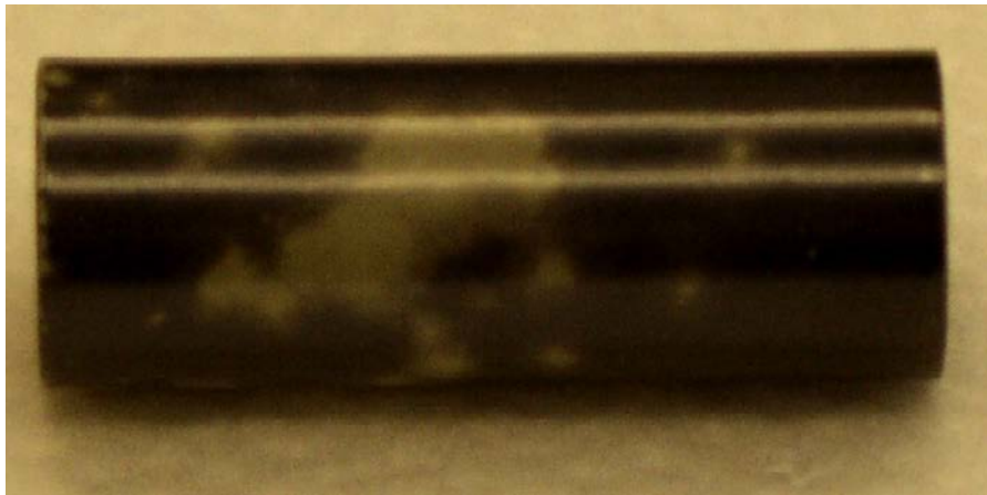
(b) W-cleaned sample #1 after 3200 s at 980°C
