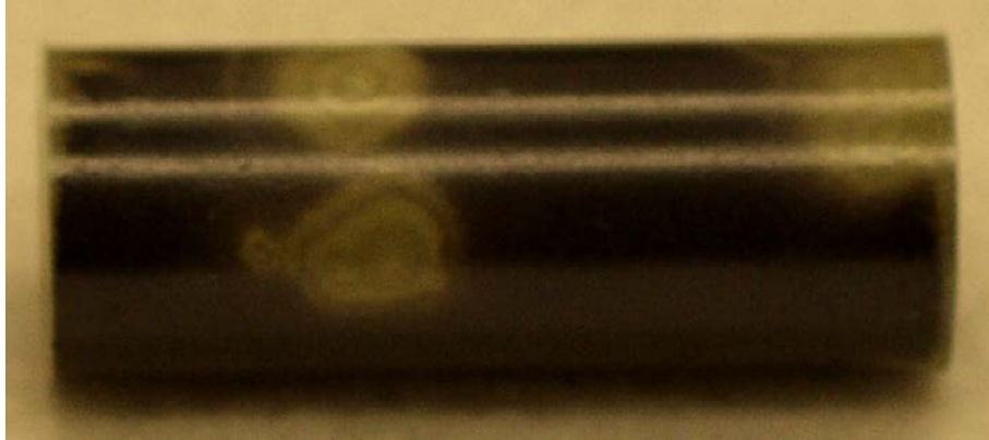
(a) ANL-cleaned sample after 3400 s at 980°C
