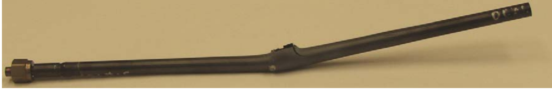
Figure 79. Post-bend appearance of the OCZL#15 sample oxidized to 18% CP-ECR, quenched, and subjected to a reverse 4-PBT with the rupture tips in compression.
