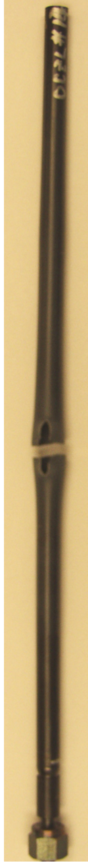
Figure E.4: Post-4-PBT images of OCZL#14 test sample, which was pressurized to 1200 psig, heated to \approx 1200^{\circ}\text{C} , oxidized to 18% CP-ECR, and cooled with quench.
