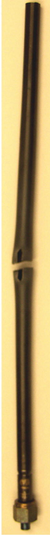
Figure E.3: Post-4-PBT image of OCZL#13 test sample, which was pressurized to 1200 psig, heated to \approx 1200^{\circ}\text{C} , oxidized to 14% CP-ECR, and cooled without quench.
