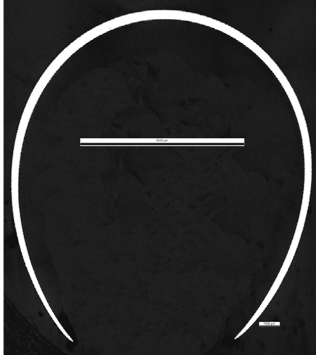
Figure 69. Rupture cross section for Studsvik Test 192 with irradiated ZIRLO pressurized to 1200 psig at 300°C. The central scale bar is 8 mm.
