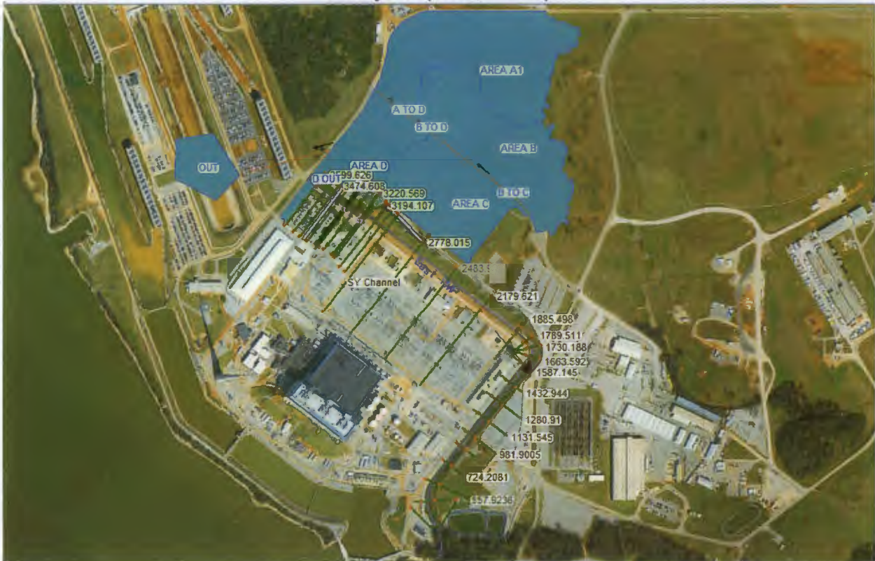
Figure 3.2-5 Layout of HEC-RAS Cross Sections and Storage Areas for the east Switchyard channel Site Drainage Analyses (NRC, 2015c)
