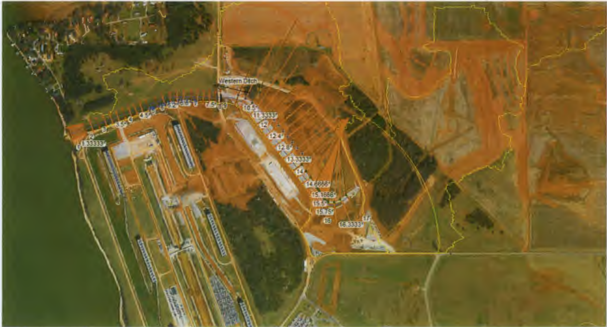
Figure 3.2-4 Layout of HEC-RAS Cross Sections for the west channel Site Drainage Analyses (NRC, 2015c)
