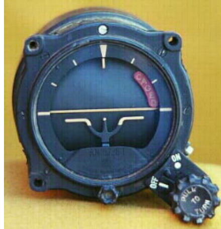
Figure 4-1. Aircraft Gauge. Certain Luminous Items Containing Radium-226 in Aircraft Are Authorized Under 10 CFR 31.12.
