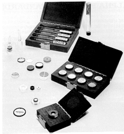
Figure 5-6. Calibration Standards. Certain calibration and reference sources containing americium-241 or radium-226 can be possessed under a general license authorized in 10 CFR 31.8 by those otherwise specifically licensed.
