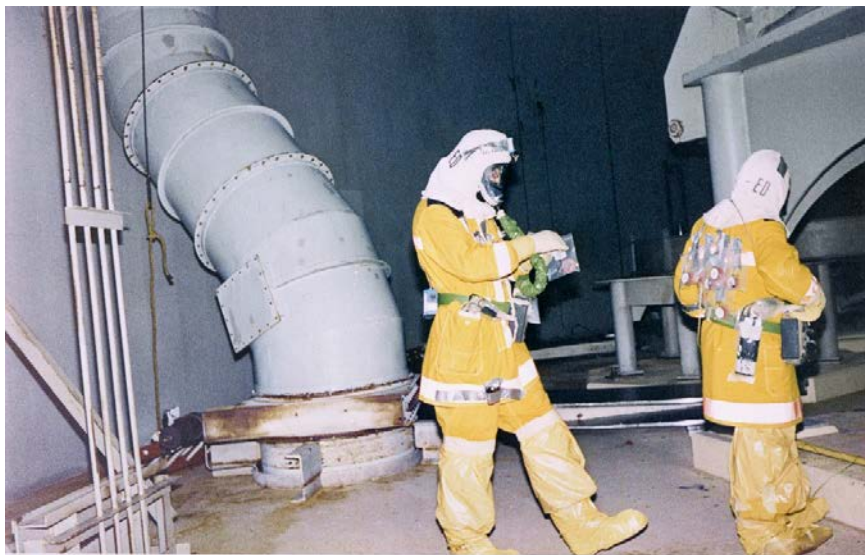
Technicians taking radiation readings inside the reactor building. Notice the personnel dosimetry attached to the back of the technician.
