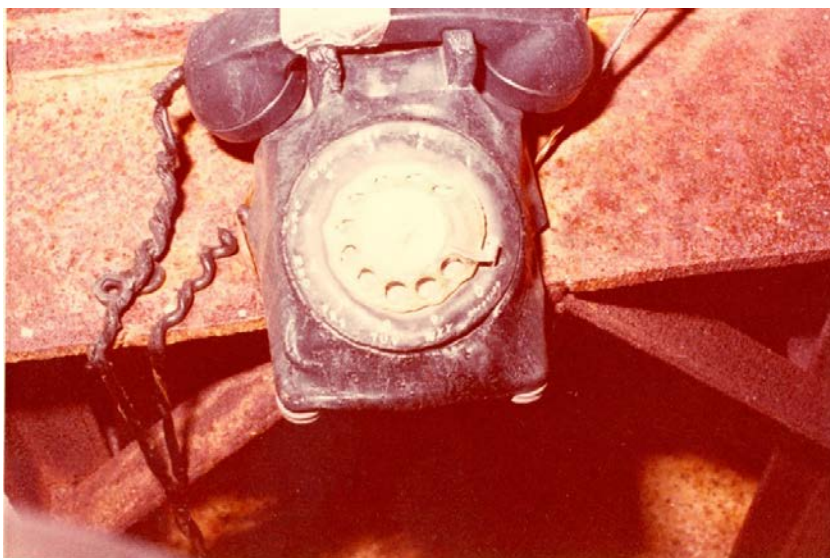
A telephone inside the reactor building during the accident was determined by INEL to sustain high temperatures from the hydrogen burn of 200 to 220 degrees Fahrenheit. The telephone case, numeral ring, and dial were distorted and the cord coils relaxed.
