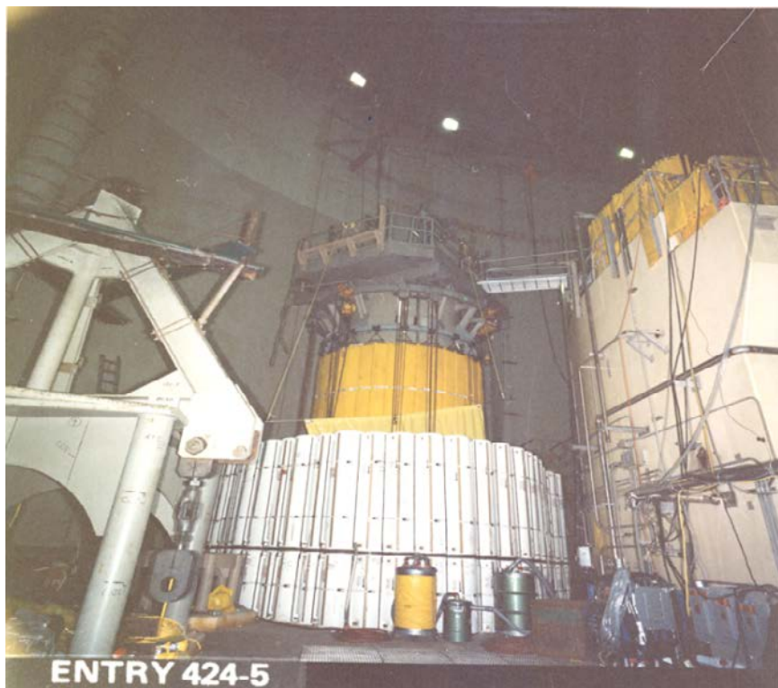
Reactor vessel head and service structure resting on its stand surrounded by shielding. Shown are white tubes filled with sand and yellow lead blankets.
