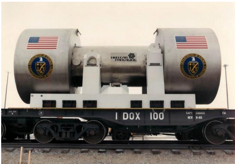
Model 125-B rail shipping cask used to transport seven defueling canisters loaded with core debris. Impact limiters shown with flags.
