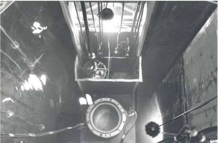
A highly radioactive spent SDS resin liner (center) being transferred into a shipping cask (lower center) while underwater in the spent fuel pool.
