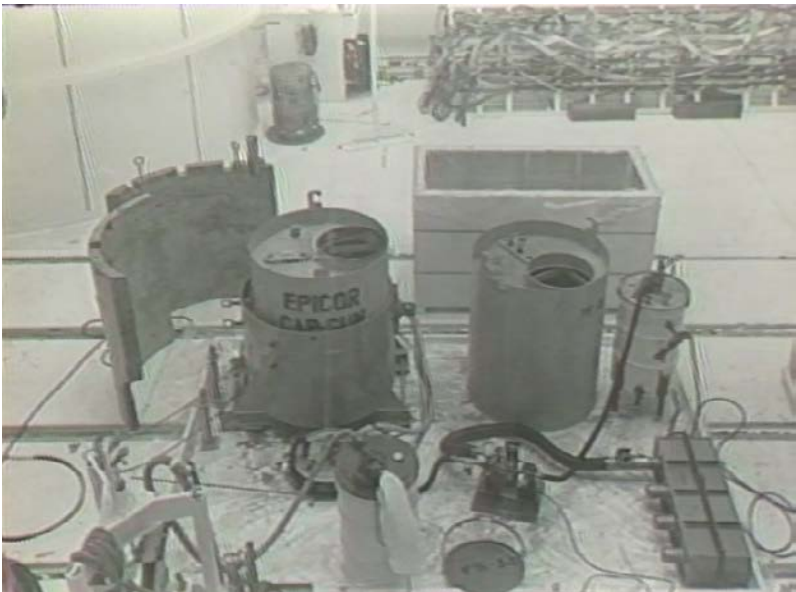
A highly-radioactive EPICOR II prefilter liner being examined in a hot cell at the Battelle Columbus Laboratory. This examination and research at other national laboratories provided information on the processing of contaminated ion exchange media and on the degradation of these media and liners.
