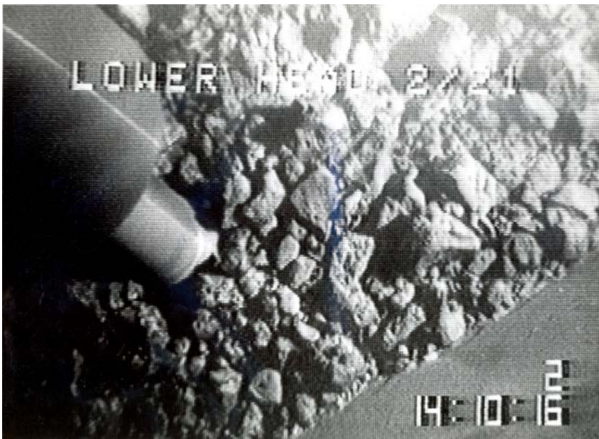
In February 1985, the first video inspection of the reactor vessel lower head region revealed a gravel-like pile of core debris. Shown left is an instrument tube penetration.
