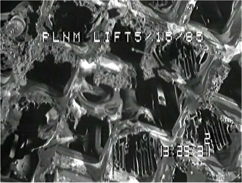
Above: Close up view of the upper grid rib section where fuel bundles were once held in place. Indication of melting of the stainless steel ribs was observed during an inspection of the underside of the upper plenum as it was lifted from the reactor vessel. Below: Broken fuel rods in the void area at the top of the damaged reactor core.
