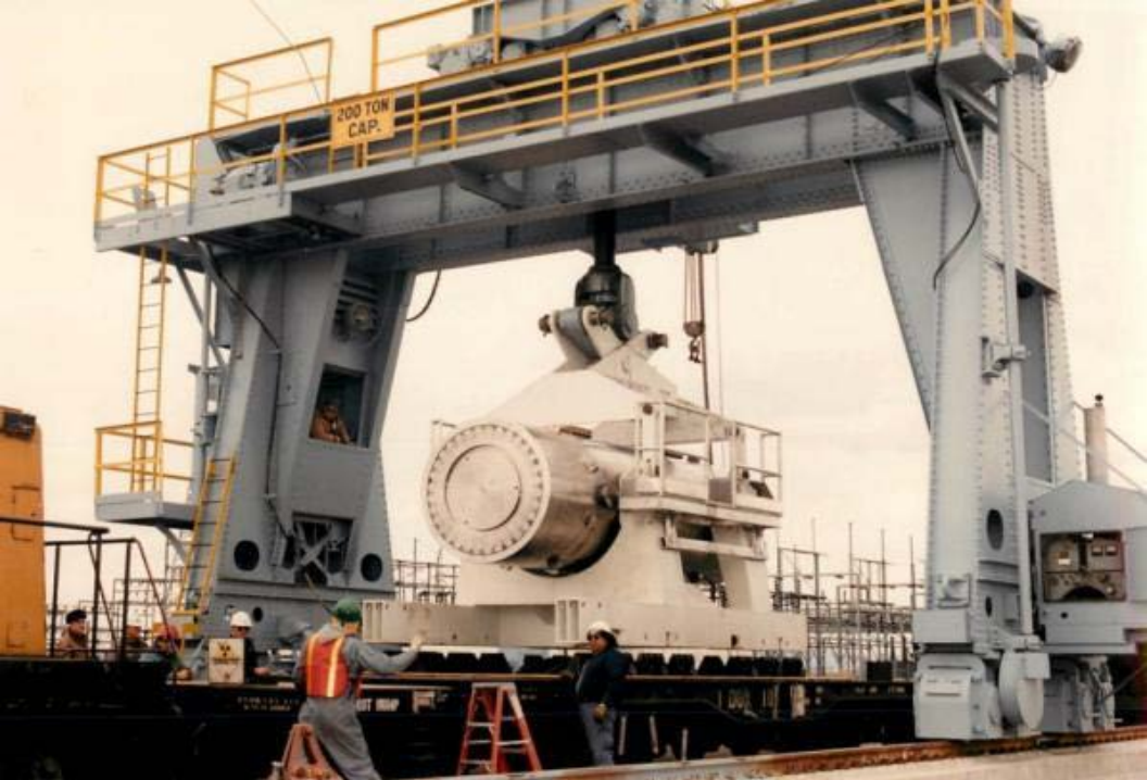
Above: The Model 125-B shipping cask being removed from the rail car at the Central Facilities Area at INEL. Both impact limiters are shown removed from the ends of the cask. Below: Defueling canisters in the temporary storage pool at INEL. A vent tube was installed on each canister for continuous venting.
