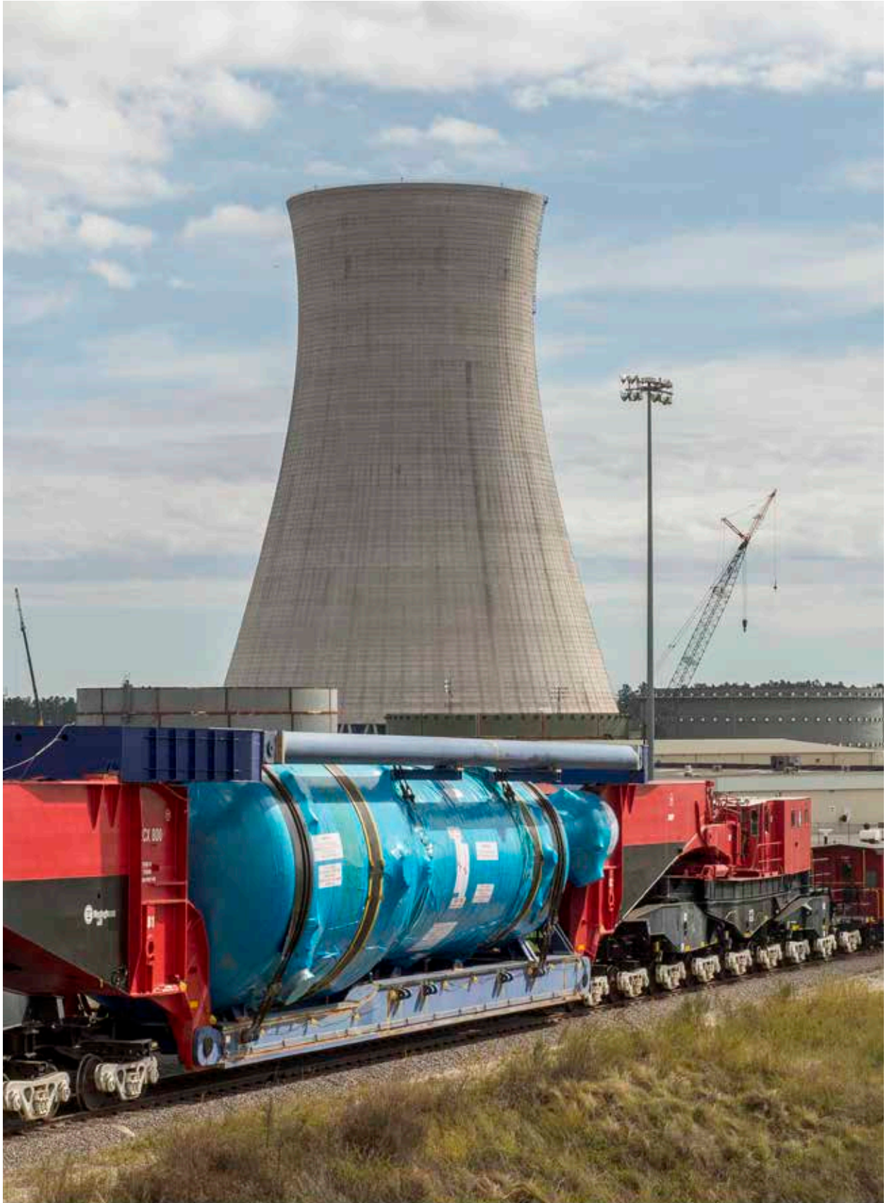
Delivery of steam generator for Vogle Unit 4. Photo courtesy of Georgia Power Company
