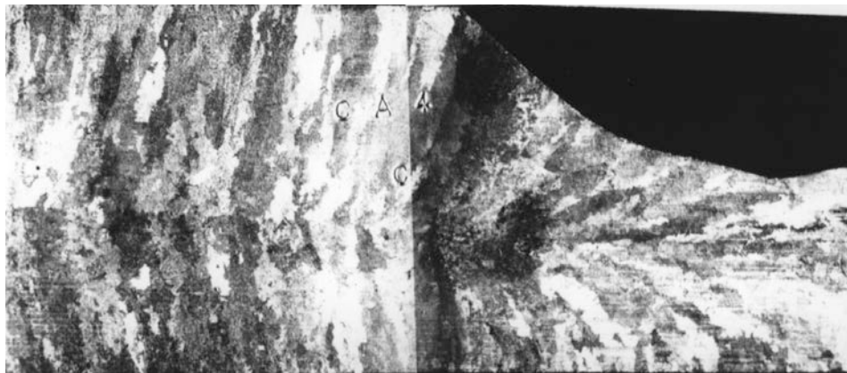
Figure 5. Microstructure along axial section of a check valve from the decommissioned Shippingport reactor showing columnar grains.
