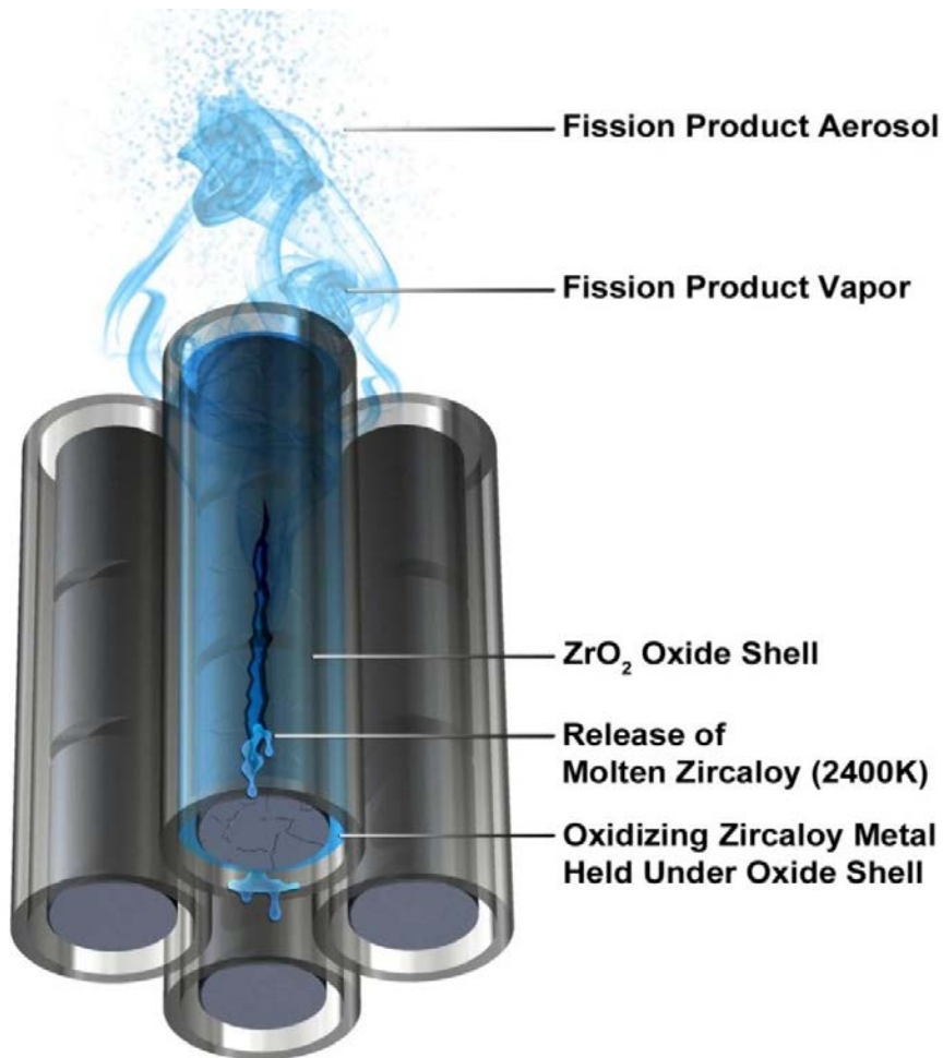
Figure 4.1-3 Depiction of the fuel rod degradation
