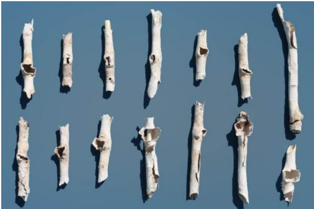
Figure 4.10 Photograph of ballooned and oxidized sections of cladding from the SFP Phase II ignition test
