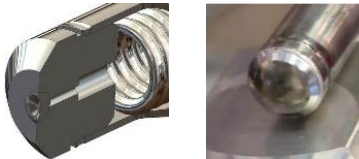
Figure 2.20 Top end plug closure weld
