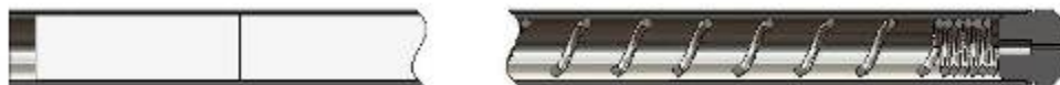
Figure 2.16 Loading of fuel rod with MgO surrogate fuel and stainless steel plenum spring
