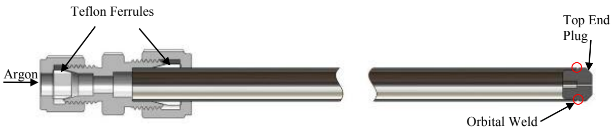
Figure 2.15 Top end plug weld setup
