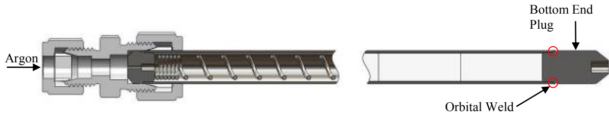
Figure 2.17 Bottom end plug weld setup
