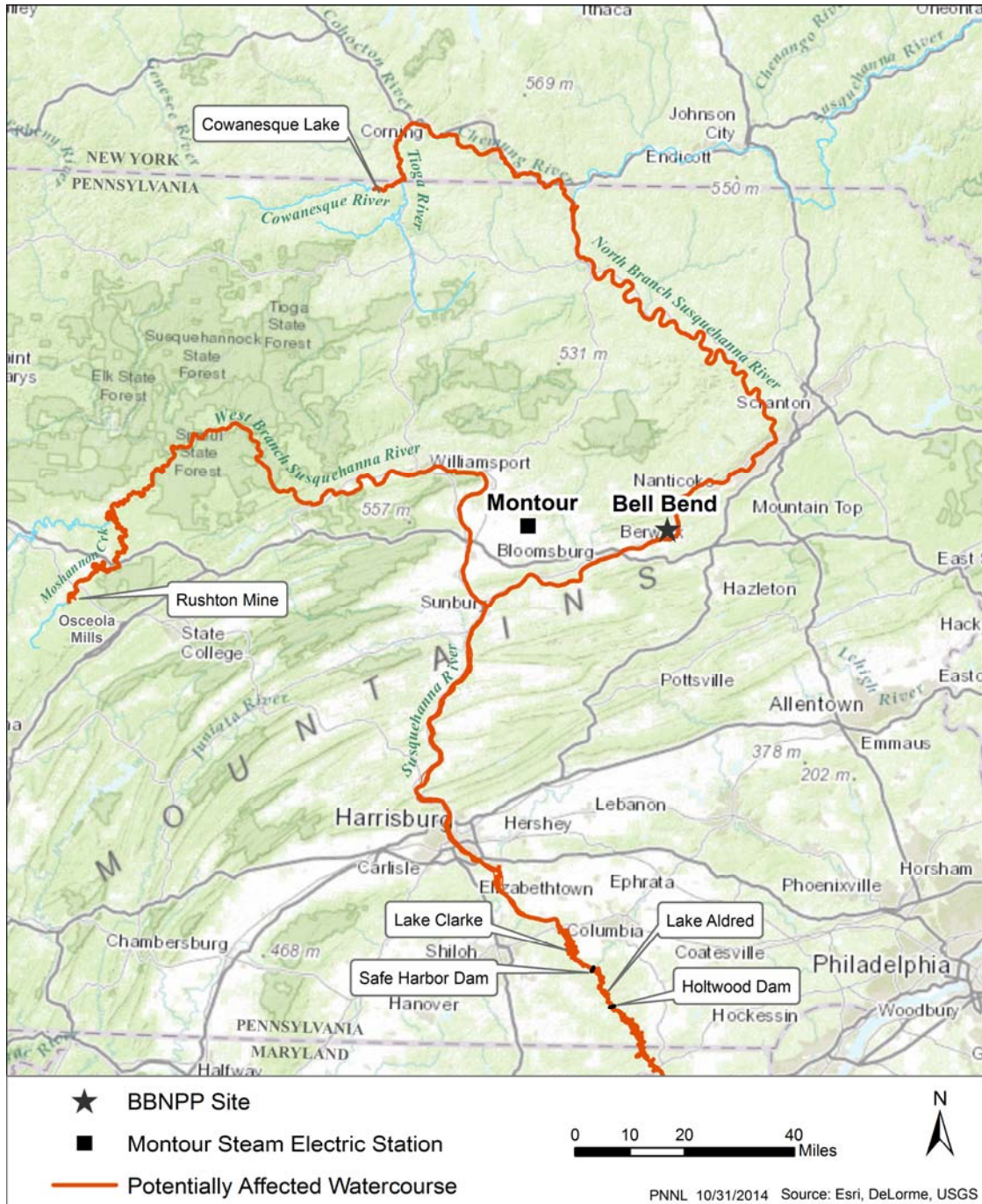
Figure 2-10. Waterbodies and Power Plants that Are Part of PPL’s Primary Plan for Consumptive-Use Mitigation and Site-Specific Low-Flow Protection
