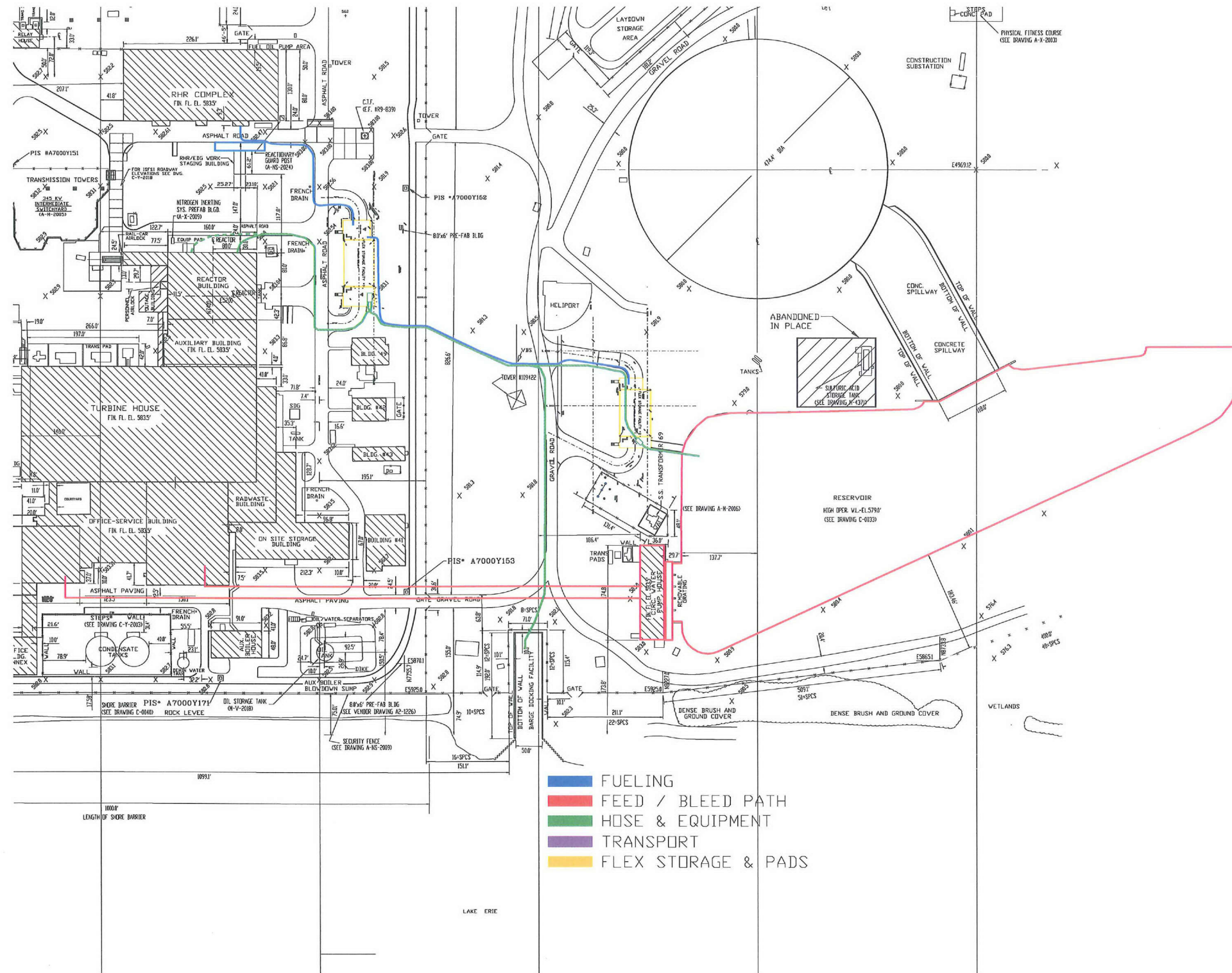
Figure 3: FLEX Deployment Paths (Inside Protected Area)
