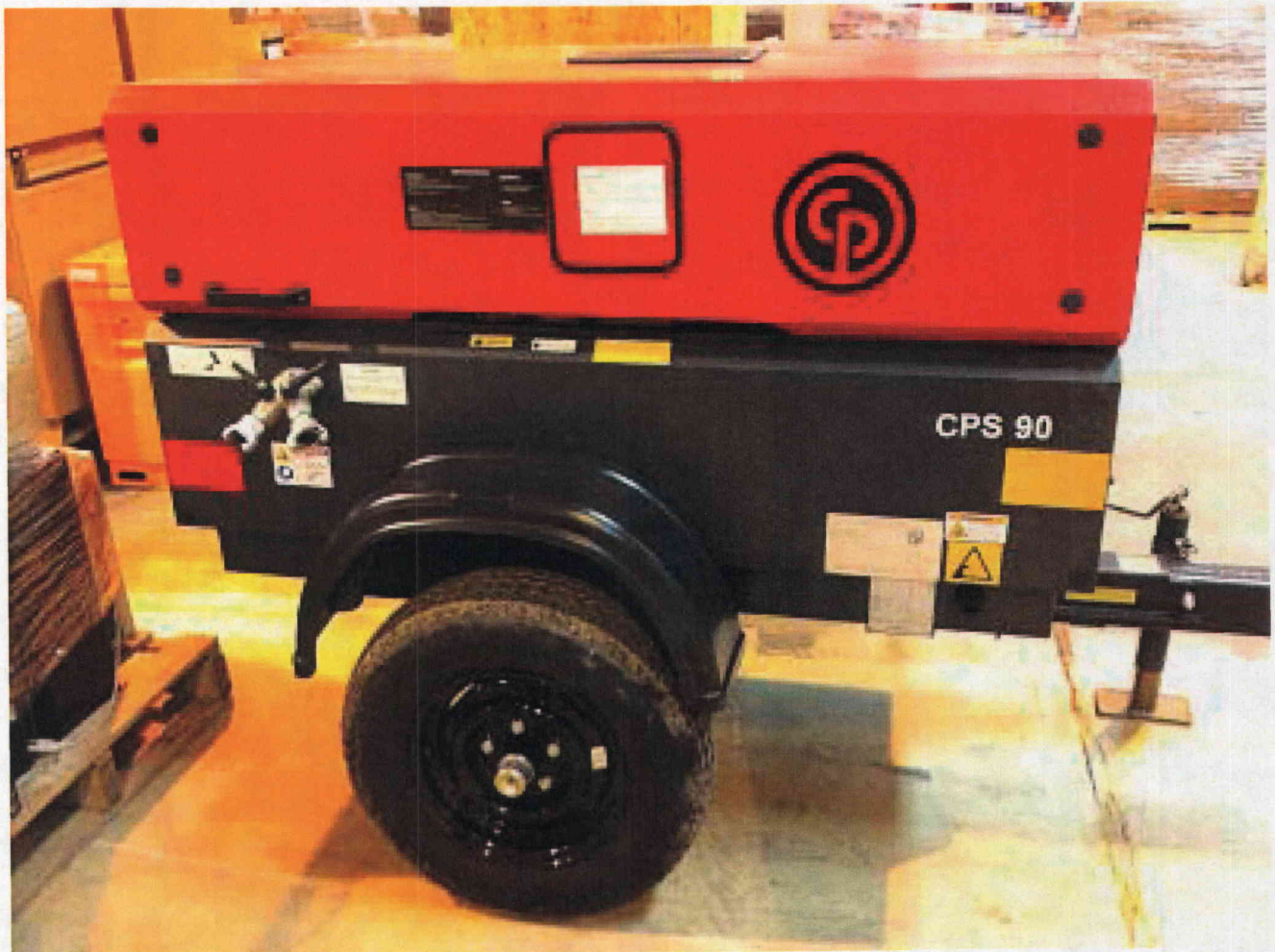
Air compressor for use in FSG 20.2 MAINTAINING ADS AIR SUPPLY
