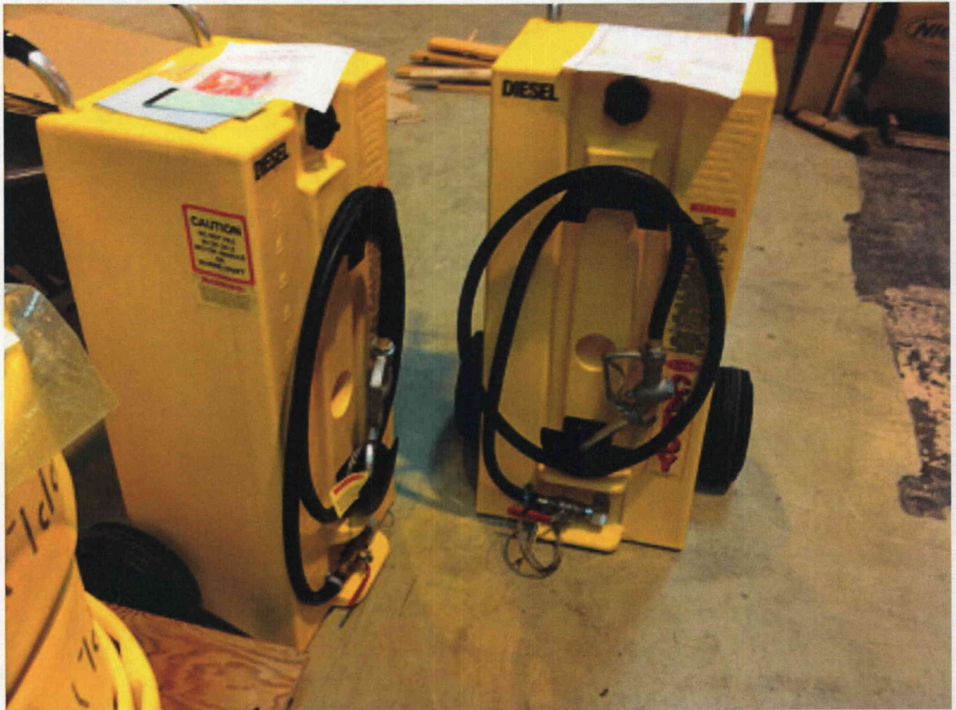
Fuel caddy for use in FSG 70.3, SUPPLYING FUEL OIL TO MISC FLEX PORTABLE EQUIPMENT
