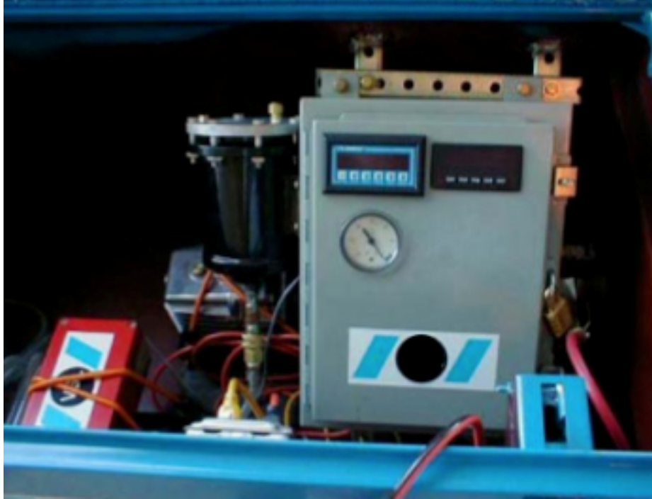
Figure 4-143 Vacuum Control and Grouting Equipment for Tendons with Defective Grouting
