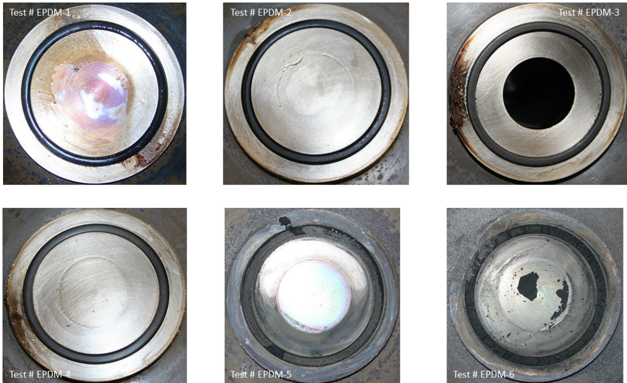
Figure 3-47. Photographs showing the thermally degraded EPDM O-ring after 8-h thermal exposure at 316 °C (600 °F) from the four EPDM O-ring tests (Tests # EPDM-1, EPDM-2, EPDM-3, and EPDM-4). Tests # EPDM-5 and # EPDM-6 were conducted at 900 °C for 9 h.
