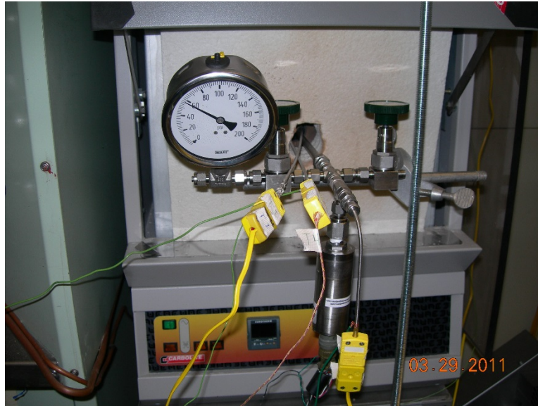
Figure 3-21. A photograph showing the pressure gauge used to check the pressure transducer performance.
