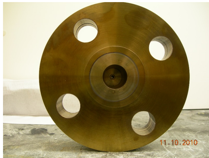
Figure 3-13. Post-test photograph of Vessel #5 (vessel body with O-ring removed) after exposure at 427 °C (800 °F) for 9 h.
