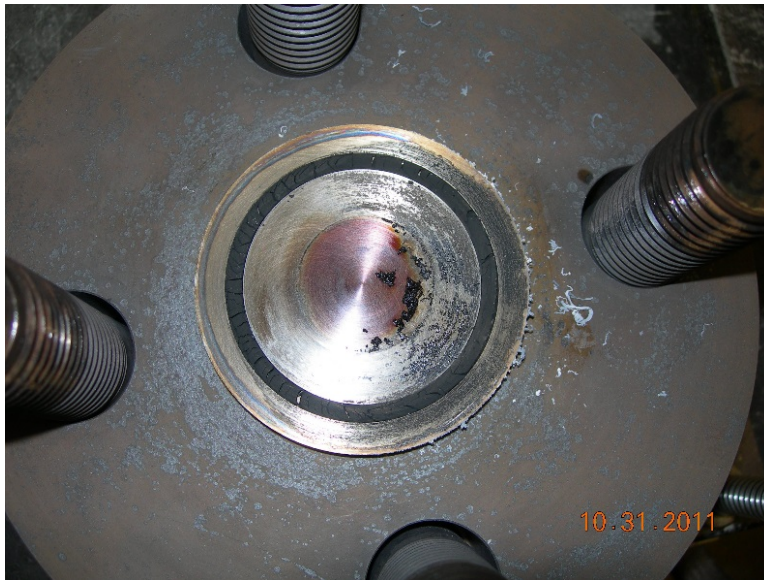
Figure 3-36. Photograph of the EPDM O-ring after thermal exposure.
