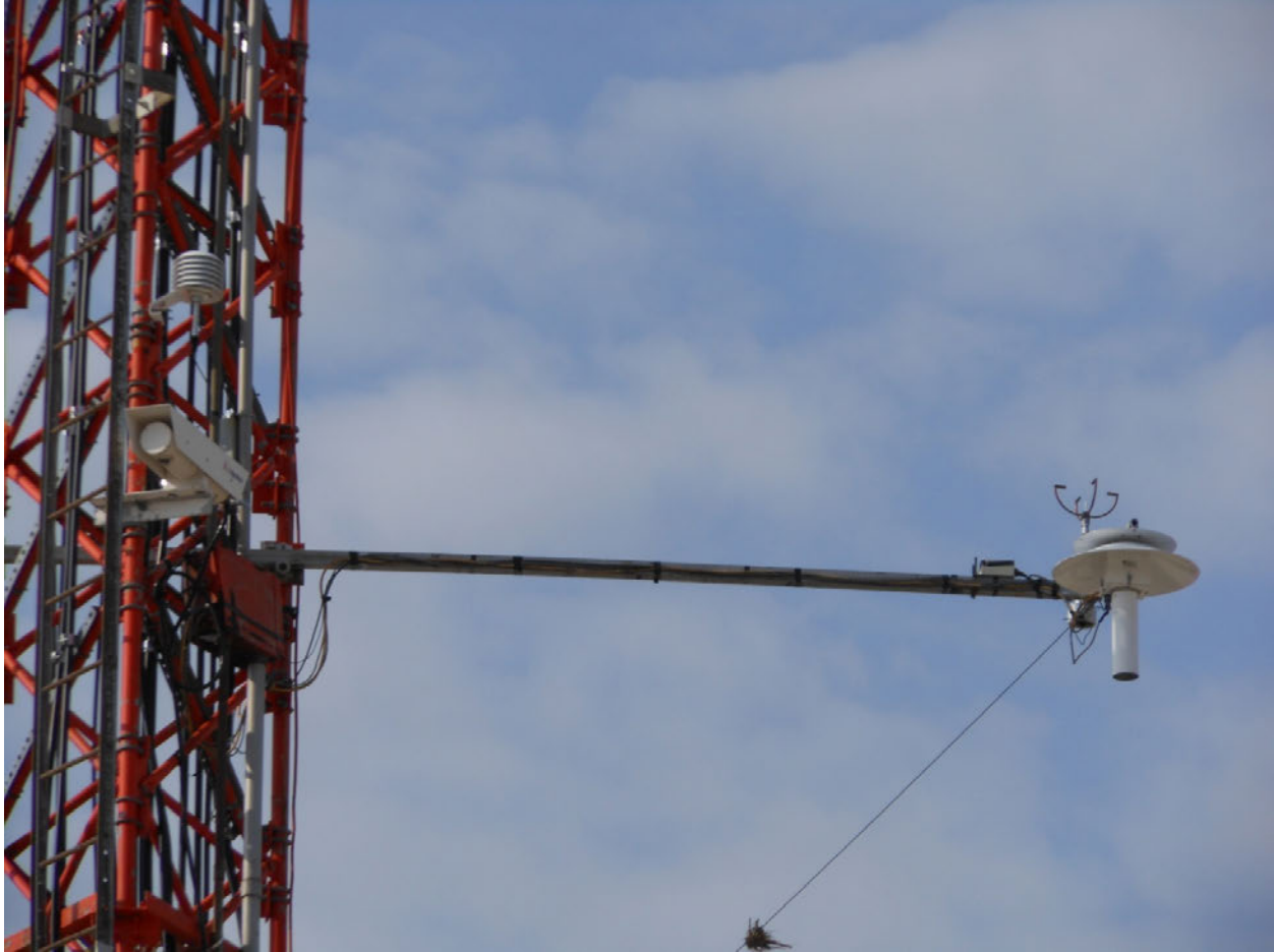
Figure 2-35. Close-up View of 33-ft Instrument Boom (dew-point sensor can be seen near top left corner of image; dry-bulb temperature, wind speed, wind direction, and delta-temperature instruments are at the end of the boom on the right side of the image) (Source: NRC staff photograph)
