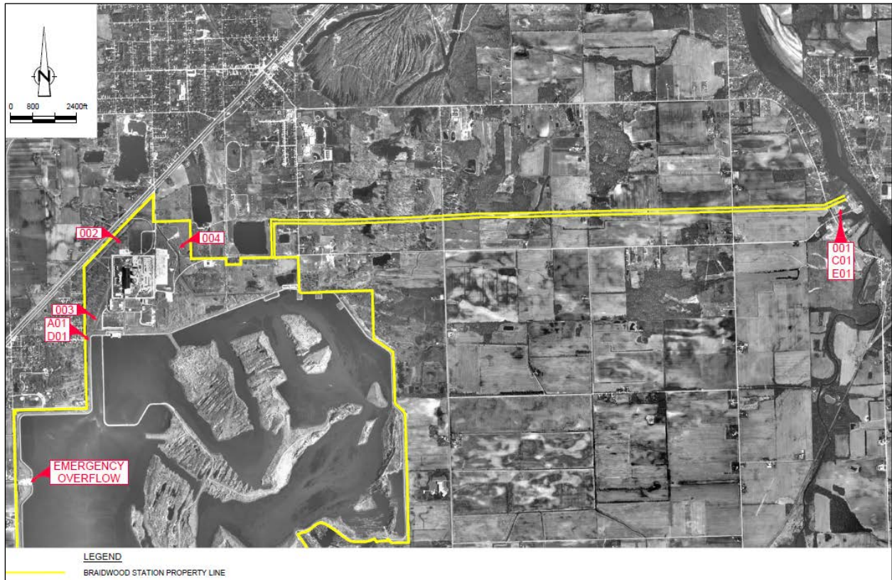
Figure 3–8. Braidwood NPDES Outfall Locations
