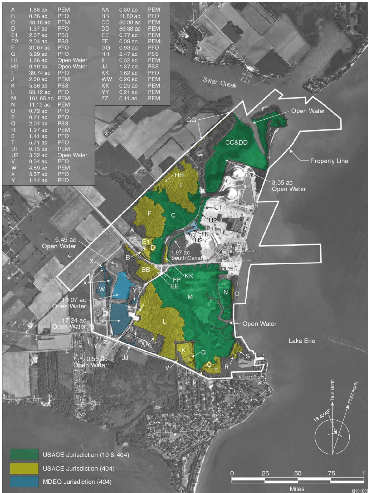
Figure 3-15. Delineated Wetlands on the Fermi Site
