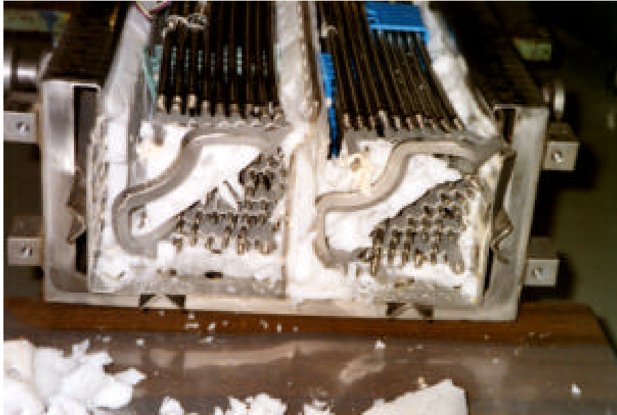
Figure 12 Photo of BWR assembly after drop test [25]
