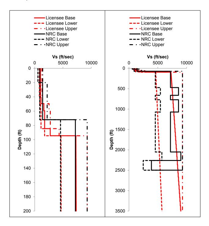
Figure 3.3-2 Plot Comparing the Staff's and the License's Median Amplification Functions and Uncertainties for two input loading levels for the Cooper Nuclear Station site
