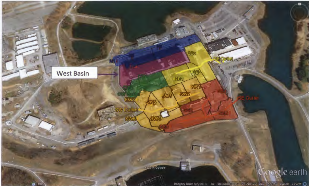
Figure 3.1-3. HEC-HMS Drainage Subbasin Model and HEC-RAS Flowpaths for Protected Area, Including the West Basin
