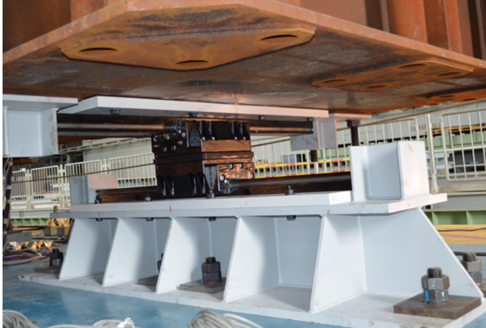
Figure 3-10 Photo of installed CL bearing illustrating orthogonal LM guides assemblies on top and bottom
