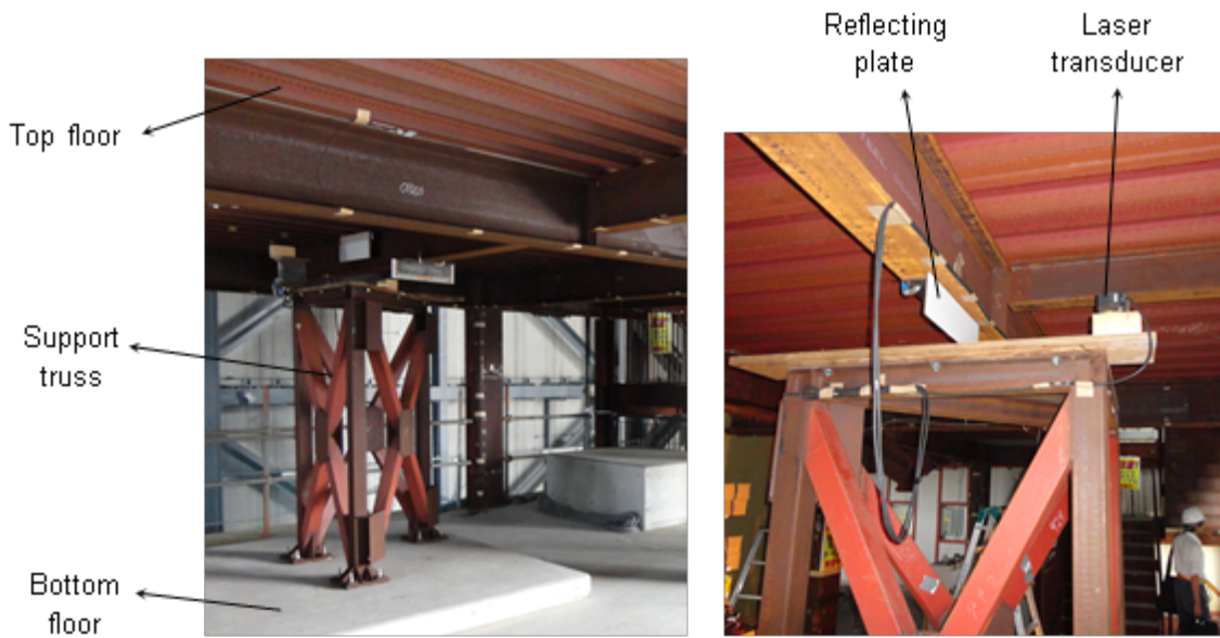
Figure 4-8 Instrumentation for measuring story drift
