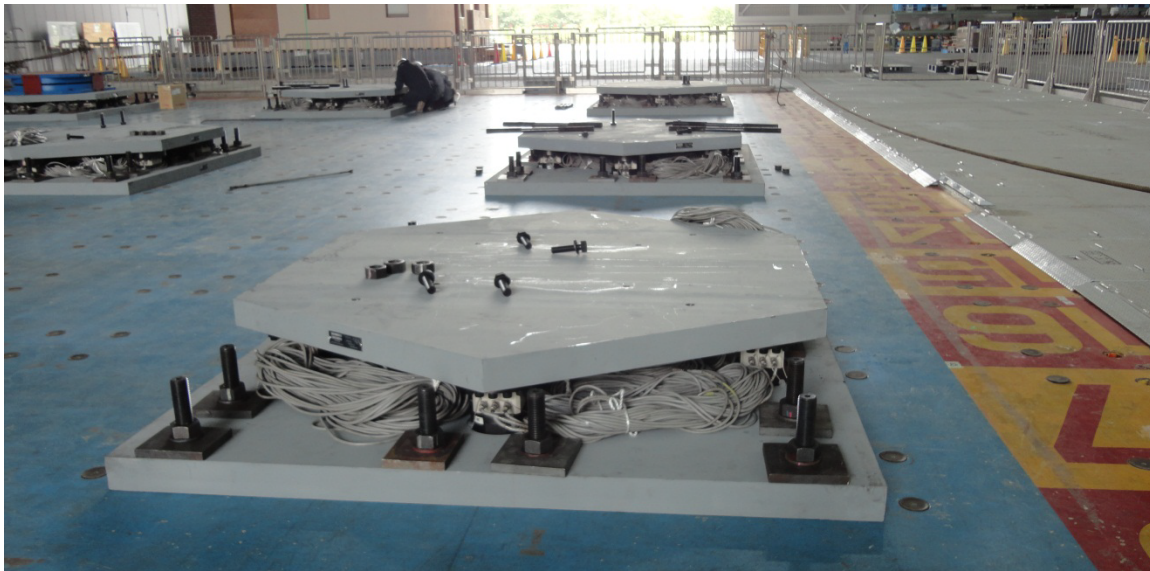
Figure 4-13 Connection assemblies on the simulator platform
