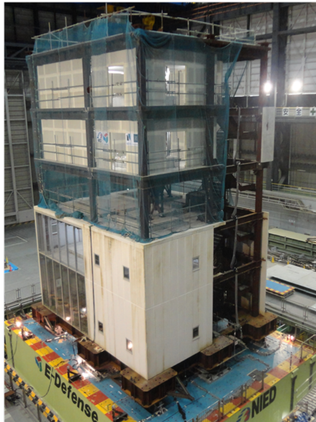
Figure 2-1 The 5-story steel moment frame specimen
