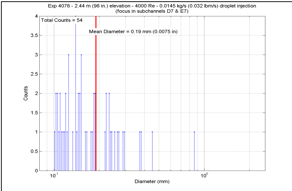
Figure A-793: Droplet Measurements at 2.438 m (96 in.) Elevation for Experiment 4076D
