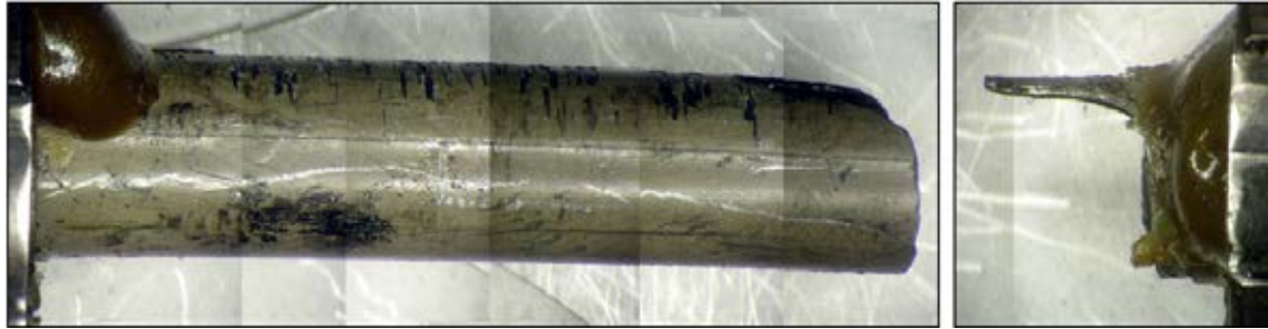
Figure 13. Mating fracture surfaces (a) and (b); lateral sides near the neutral axis of the bending rod for S1 (606C3C) (c) and (d). The rod was subjected to four repeat static cycles to 24 mm maximum relative displacement followed by dynamic cyclic loading \pm 25.40 to 30.48 N·m at 5 Hz; 1.4 \times 10^4 failure cycles, 0.9 gram fuel particles collected. Note: This specimen appears to have been loaded into the test machine at 90^\circ off from the ID marks
