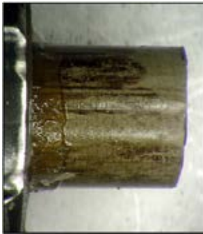
Figure 24. (a) and (b) Mating fracture surfaces, (c) frontal, and (d) back sides for D1 (607C4B), N_f = 1.1 \times 10^5 cycles under \pm 15.24 N·m, 5 Hz. Fuel particles collected < 1.0 g.
