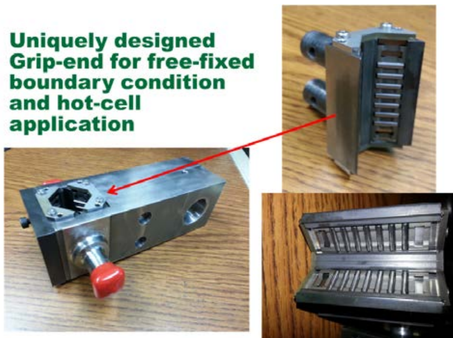
Figure 3. Assembled grip (left) and two views (right) of detached grip body.
