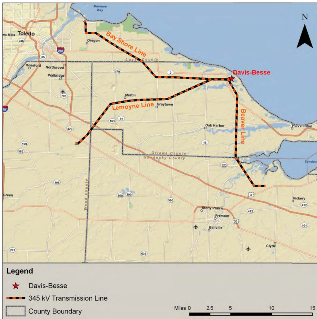
Figure 2–6. Davis-Besse Transmission System
