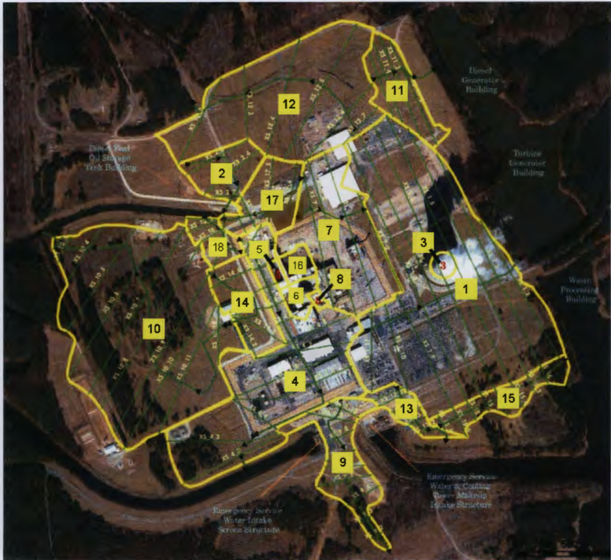
Figure 3.2-1. Locations of Buildings, Subbasins, and Cross Sections in the HNP Unit 1 Site Hydraulic Model
