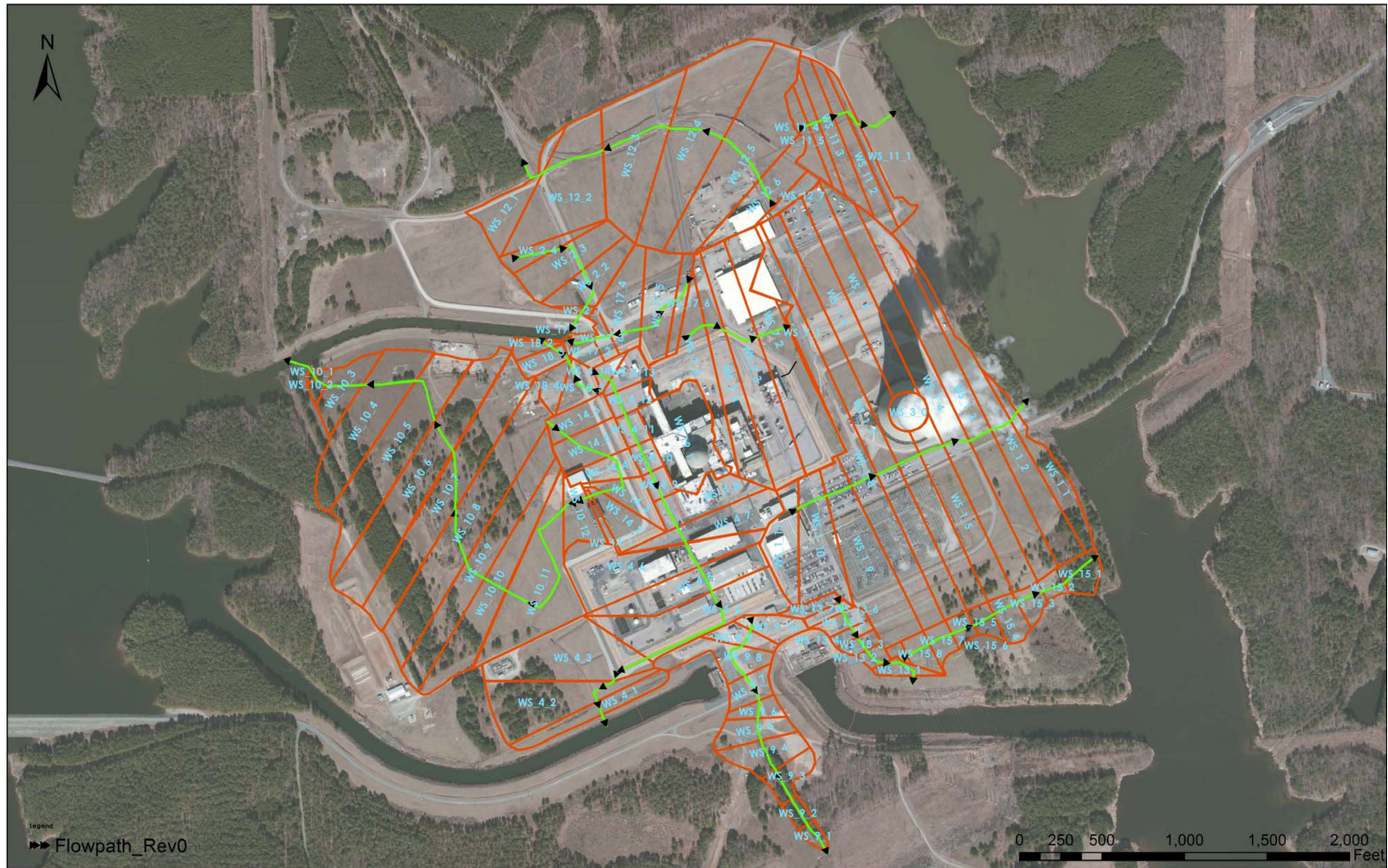
Figure 2. Delineated watershed for the HNP site with contributing area for each cross-section
