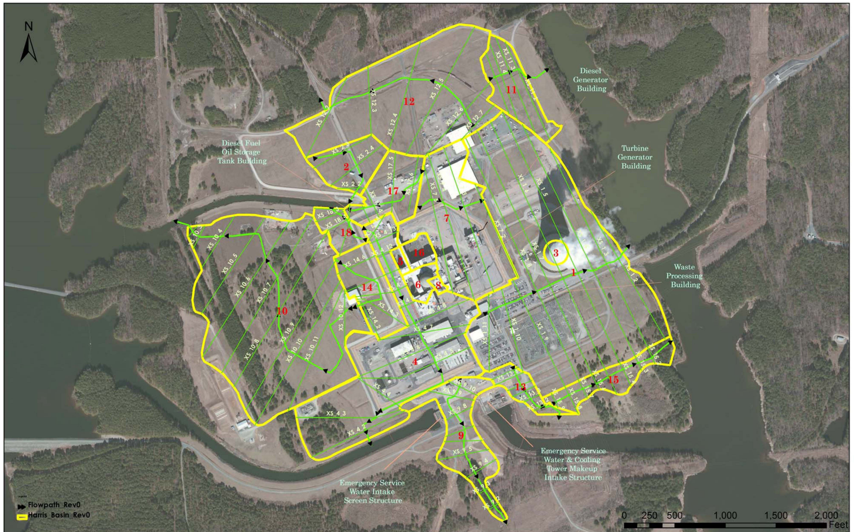
Figure 3. Delineated watershed for the HNP site with cross-sections and location of safety-related structures and buildings
