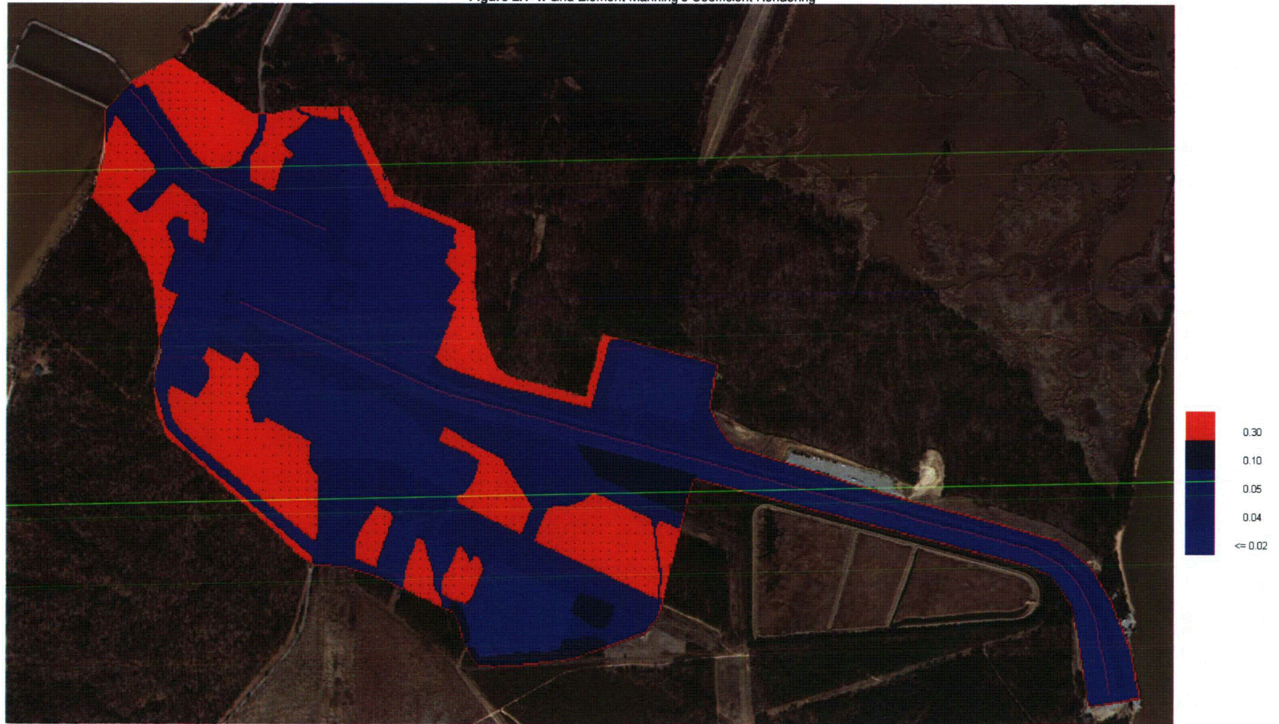
Figure 2.1-4: Grid Element Manning's Coefficient Rendering
