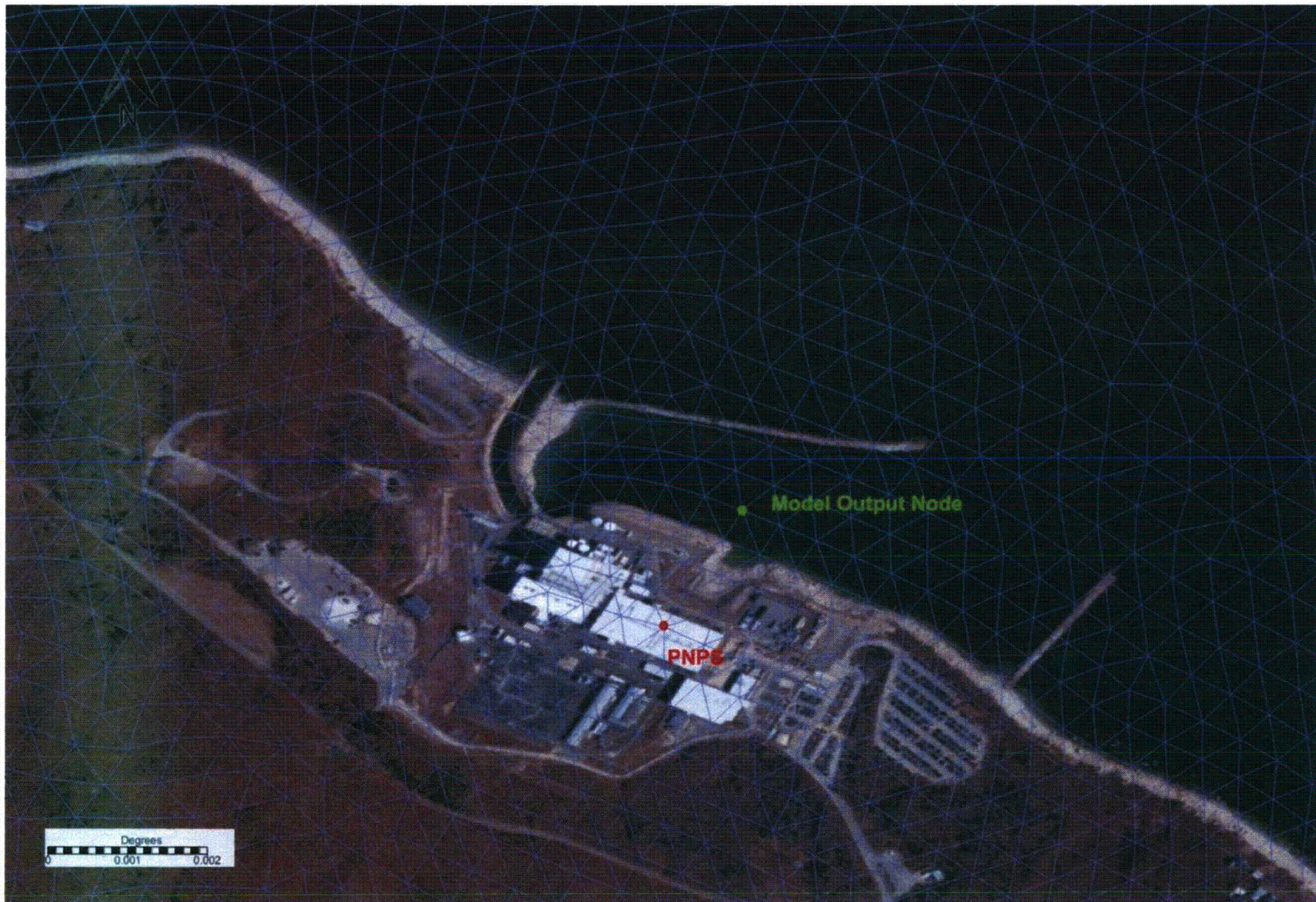
Figure 3-28: ADCIRC/ADCIRC+SWAN Finite Element Mesh for PNPS – PNPS Vicinity
