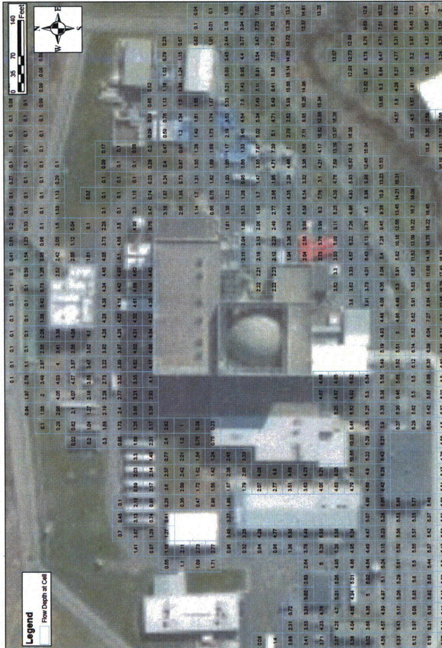
Figure 13: Probable Maximum Flow Depths at Ginna (ft, NGVD29) (Combination of PMF on Deer Creek and 25-year Surge with wind-wave activity and the maximum controlled water level in Lake Ontario)
