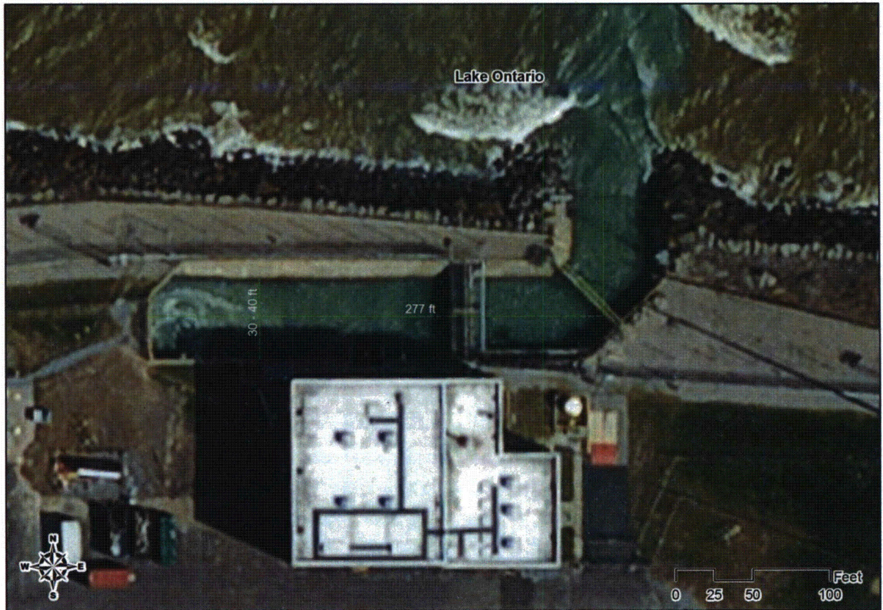
Figure 2.5-1: Discharge Canal Dimensions
