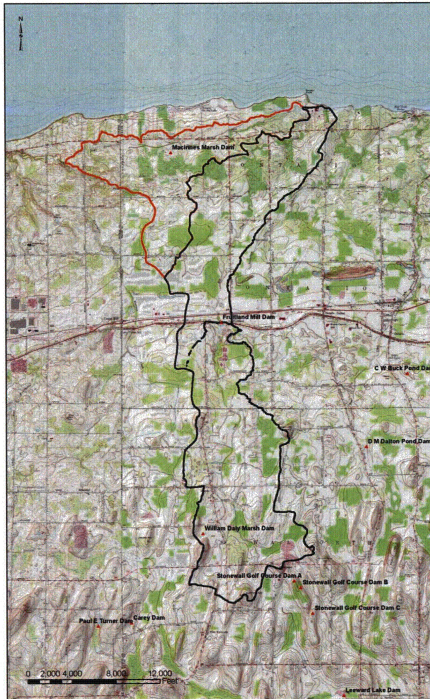
Figure 2.3-1: Watershed Delineation and Dam Locations
