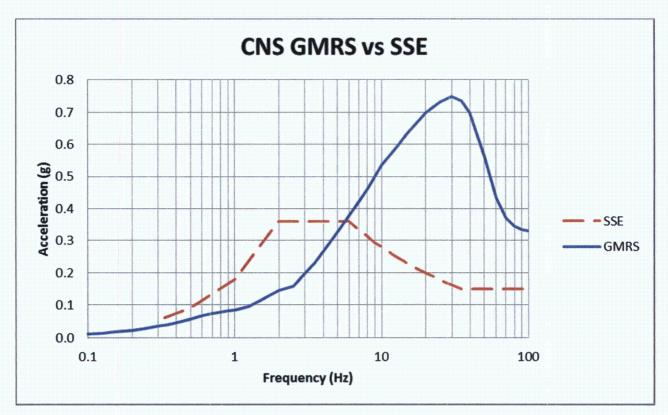
Figure 4-4. Comparison of CNS GMRS and SSE (5% Damping).
