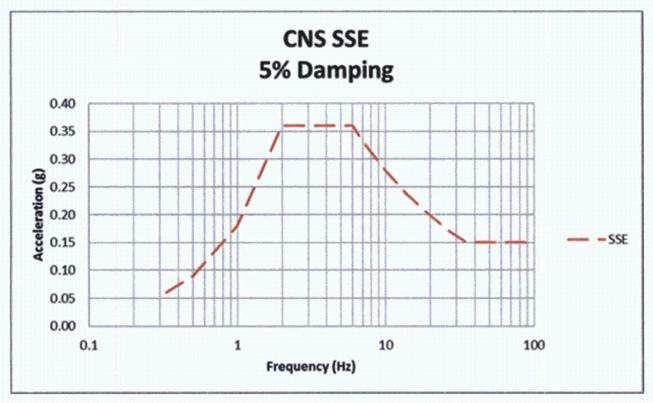
Figure 4-3. CNS SSE (5% Damping).
