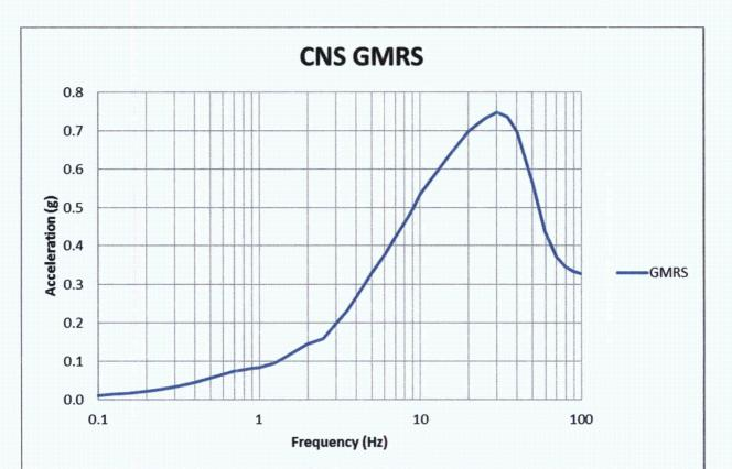
Figure 4-2. CNS GMRS (5% Damping) – Graphical Form [4].
