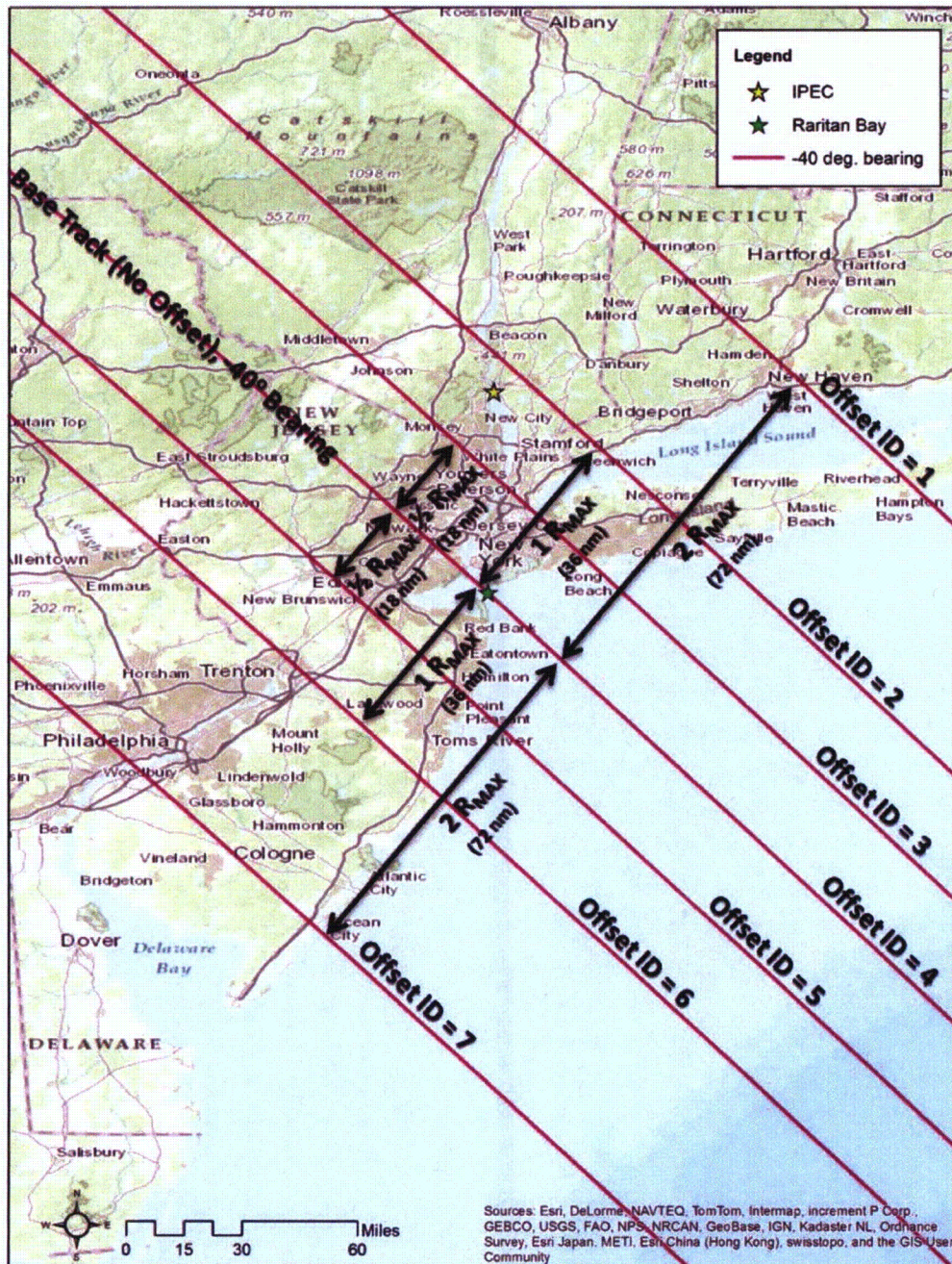
Figure 3.4-32: Example Storm Tracks ( \theta =-40 degree bearing) with Offset Calculation (Offset IDs Indicated) from Base Track (AREVA, 2013e)
