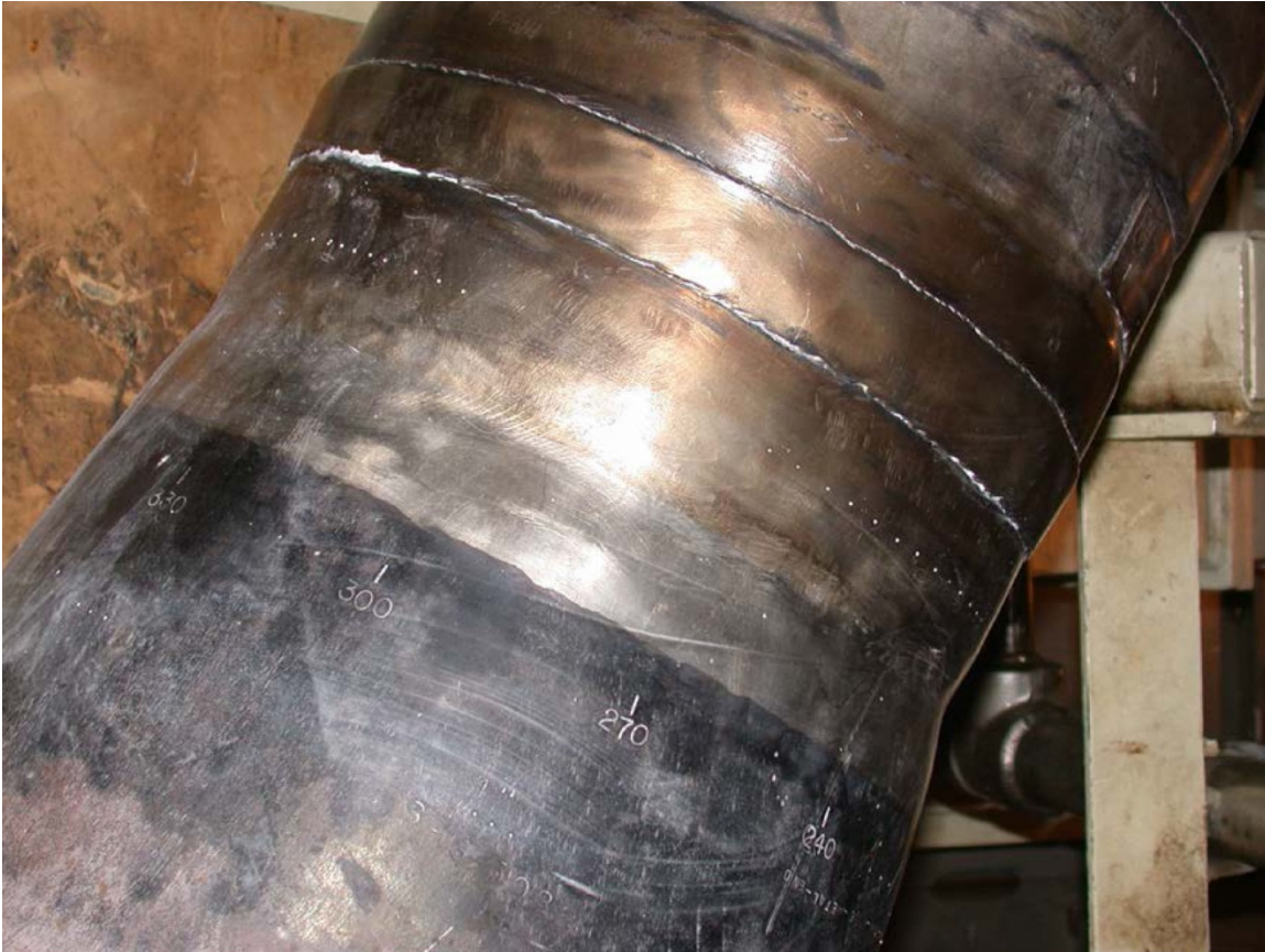
Figure D.20 Photograph of Safety Injection Nozzle, Nozzle Weld, and Safe End
