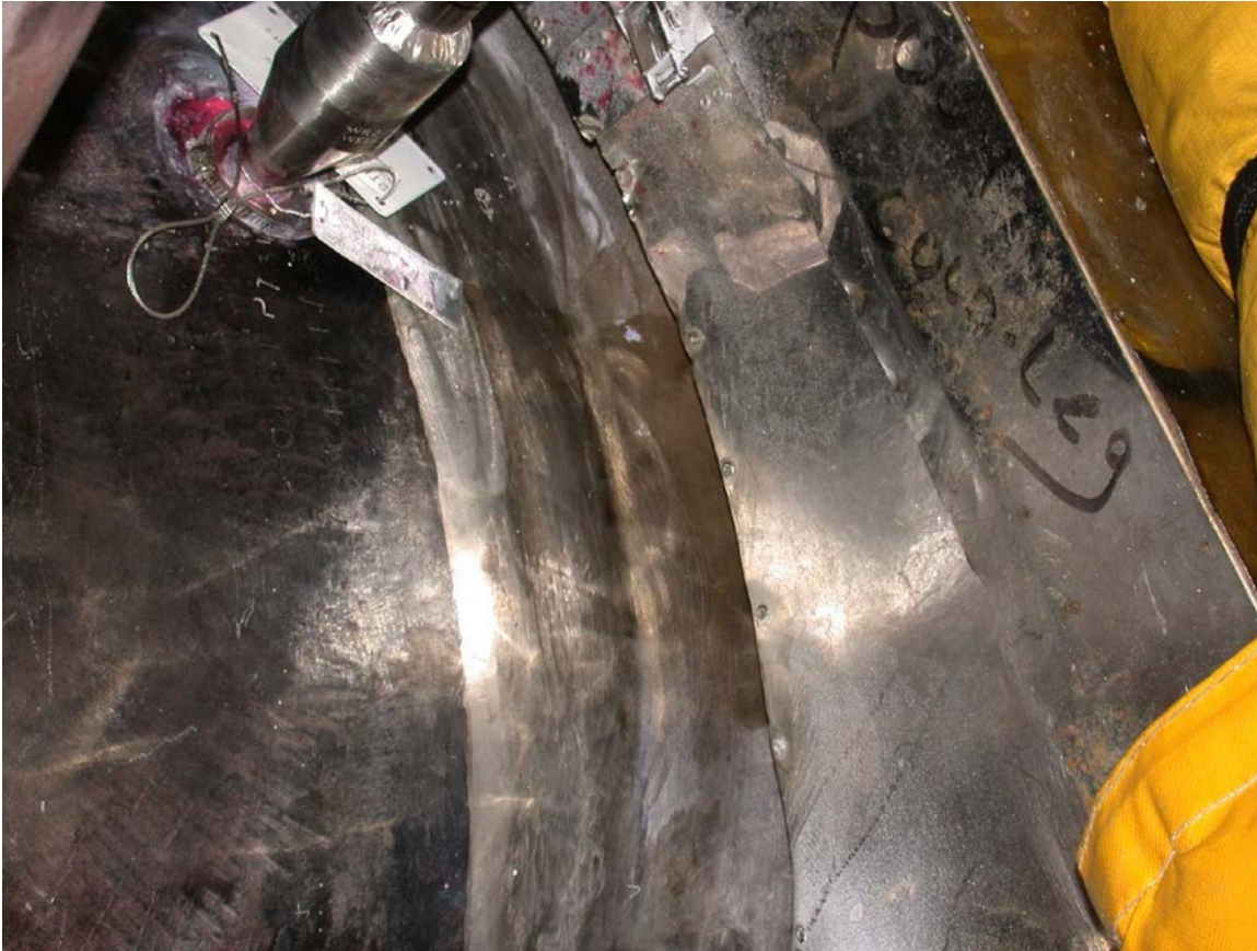
Figure D.5 Photograph of RCP Discharge Nozzle, Nozzle Weld, and Safe End
