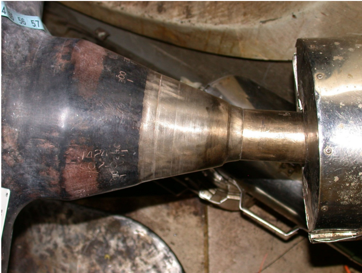
Figure D.17 Photograph of Charging Inlet Nozzle, Nozzle Weld, and Safe End
