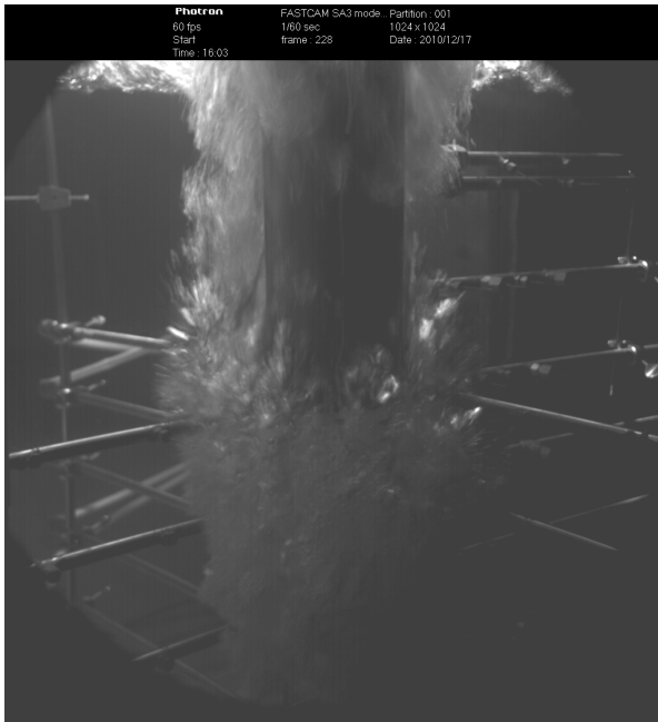
Figure 4-23 Bubble Plume Around the Downcomer Exit During t=3.13-3.93 Seconds for Test No. T5 (Based on the High-speed Camera Time)
