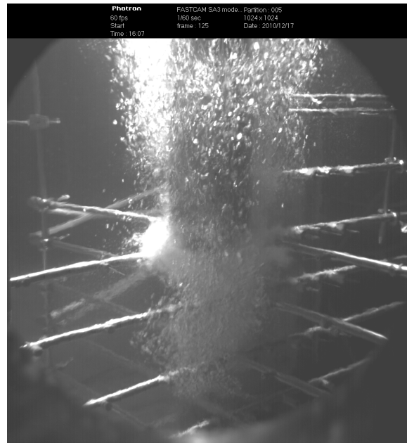
Figure 4-26 Bubble Plume Around the Downcomer Exit During t=300 and 542.08 Seconds for Test No. T5 (Based on the High-speed Camera Time)
