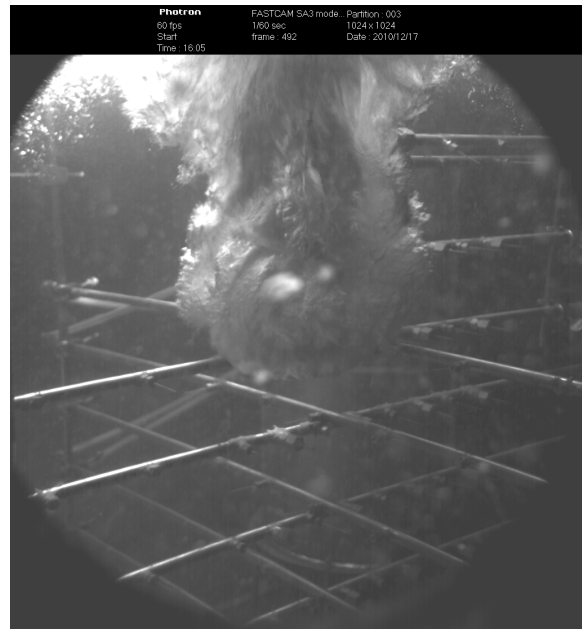
Figure 4-25 Bubble Plume Around the Downcomer Exit During t=31.93 and 68.20 Seconds for Test No. T5 (Based on the High-speed Camera Time)
