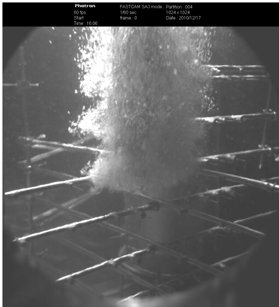
Figure 4-26 Bubble Plume Around the Downcomer Exit During t=300 and 542.08 Seconds for Test No. T5 (Based on the High-speed Camera Time)
