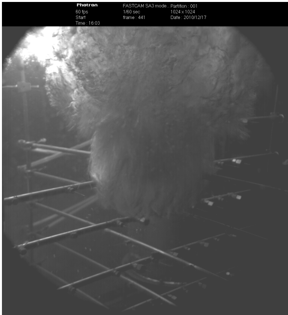
Figure 4-24 Bubble Plume Around the Downcomer Exit During t=5.10-7.48 Seconds for Test No. T5 (Based on the High-speed Camera Time)
