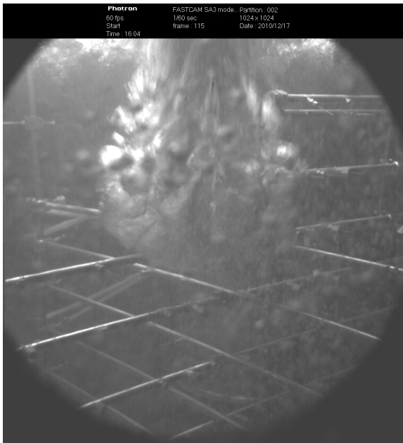
Figure 4-25 Bubble Plume Around the Downcomer Exit During t=31.93 and 68.20 Seconds for Test No. T5 (Based on the High-speed Camera Time)
