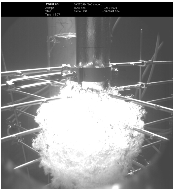
Figure 4-1 Bubble Plume Around the Downcomer Exit During t=1.084-1.420 Seconds (the Initial Period) for Test No. A1
