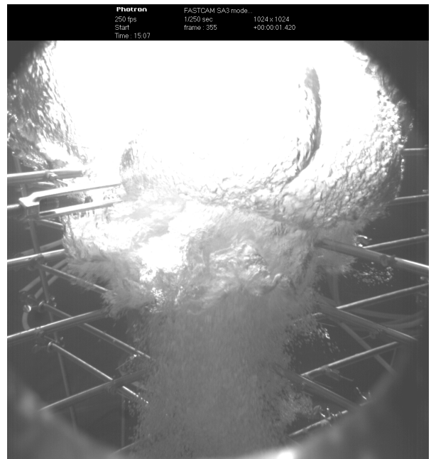
Figure 4-1 Bubble Plume Around the Downcomer Exit During t=1.084-1.420 Seconds (the Initial Period) for Test No. A1
