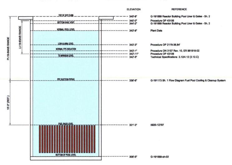
FIGURE 1 (SFP Elevation View with Levels Indicated)
