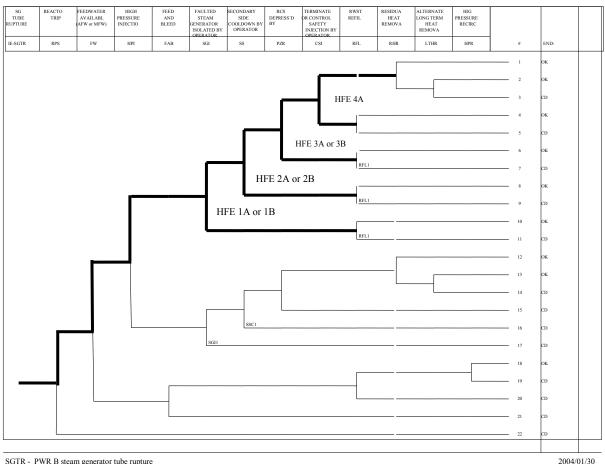
SGTR - PWR B steam generator tube rupture
