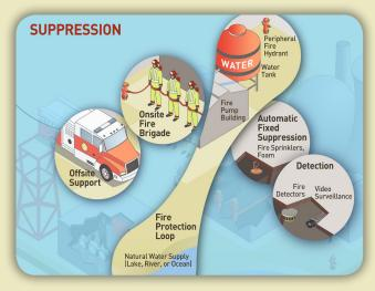
• Automatic Fixed Fire Sprinklers, Foam—Plants' installed firefighting systems operate automatically to control and extinguish plant fires. These general area protection systems are usually fire sprinklers. Special hazards such as oils can require foam-based systems.
