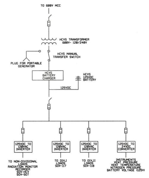
Sketch 1.A: Electrical Layout of System – One Line Diagram
