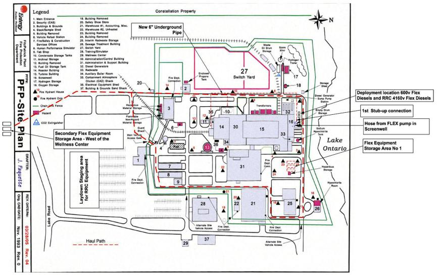
Sketch 3.C: Plant Layout – Deployment Location and Travel Path (From FLEX OIP; Ref. 28)
