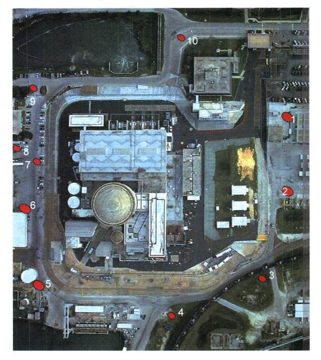
Figure I-5: CR3 Groundwater Monitoring Well Locations Deep Wells Are Also Installed at #'s 1, 3, 6
