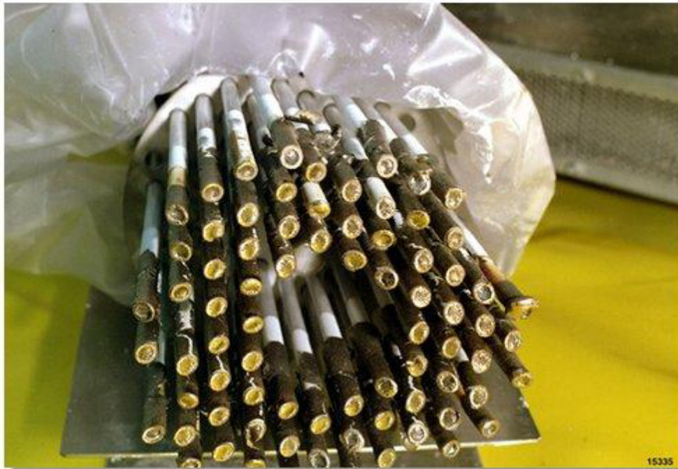
Figure C.27 Metal fuel after casting
