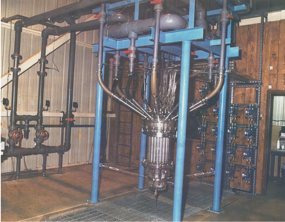
Figure C.51 Core flow test with water (SP-100 LMR)
