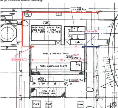
Figure 1: SFP Plan View
