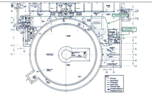
Figure 2.1.4-2 - Modes 5 & 6 Core Cooling & Heat Removal FLEX Strategy - 1974' El. (Ref. 6.3.3)
