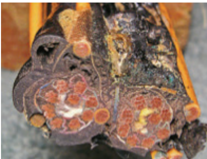
Picture of damaged cables resulting from an Electric Power Research Institute (EPRI) cable fire test
