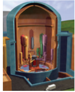
U.S. EPR containment Courtesy: AREVA NP
