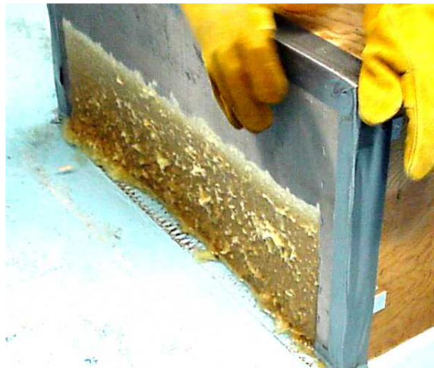
Figure 5.4-7. Typical Accumulation of Fine Fibrous Debris (Figure 6-7 in NUREG/CR-6773)
