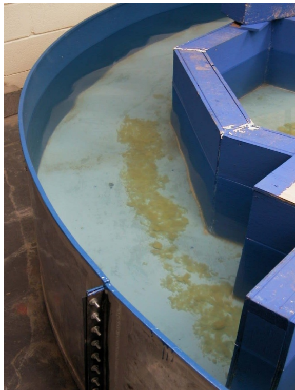
Figure 5.4-6. Debris Stalled in a Slow-Flowing Region of the Simulated Annulus (Figure 6-3 in NUREG/CR-6773)
