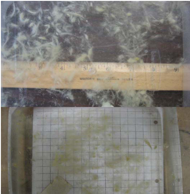
Figure 5.11-4. Photograph of GE Prepared Fibrous Debris (OPPD 2008)
