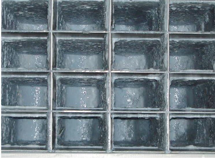
Figure 5.7-6. Thin-bed on CCI Pocket Strainer Design
